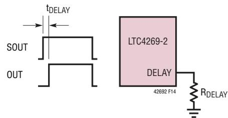
Figure 14. Programming SOUT and OUT Delay:  $t_{DELAY}$
