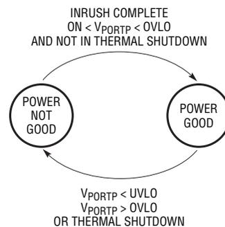
Figure 6. LTC4269-2 Power Good Functional and State Diagram
