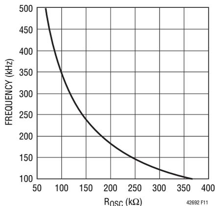
Figure 11. Oscillator Frequency,  $f_{OSC}$ , vs  $R_{OSC}$
