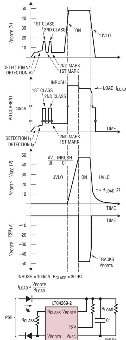
Figure 4. V<sub>NEG</sub>, T2P and PD Current as a Result of 2-Event Classification
