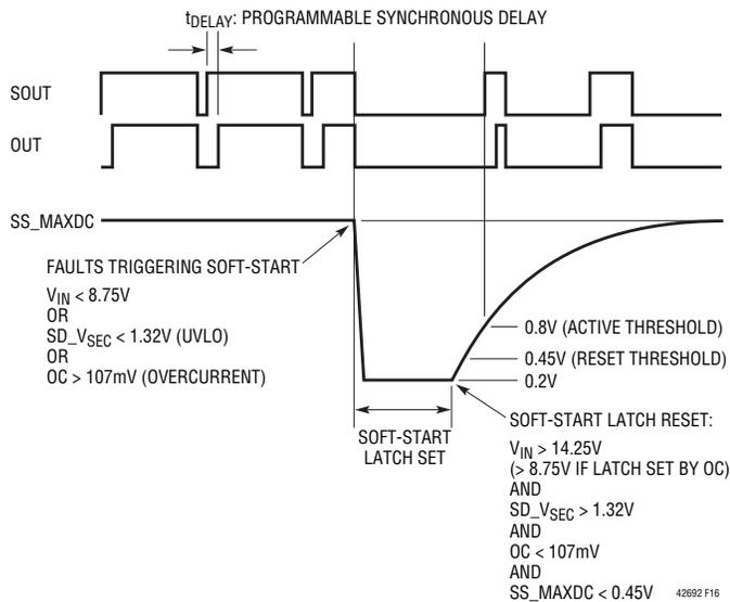
Figure 16. Timing Diagram
