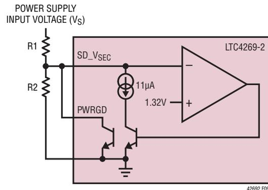
Figure 9. Programming Power Supply Undervoltage Lockout (UVLO)
