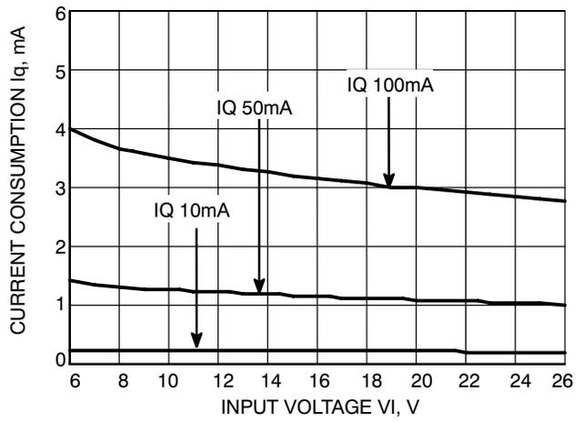
Figure 17. Current Consumption Iq vs. Input Voltage VI
