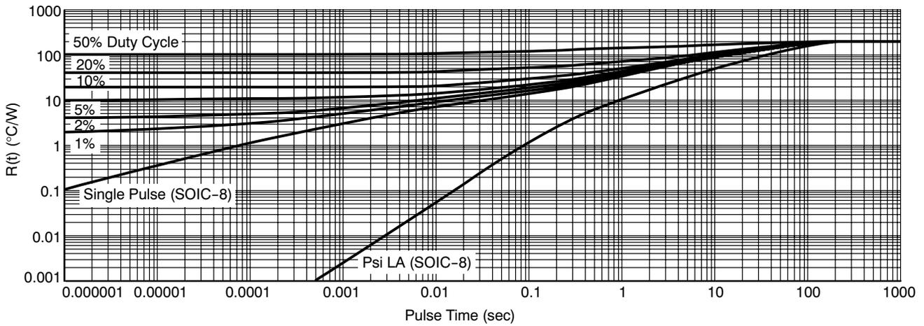
Figure 45. Transient Thermal Response Simulation to a Single Pulse with Duty Cycles Applied (Log-Log)
