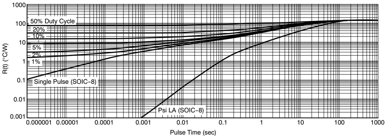
Figure 46. Transient Thermal Response Simulation to a Single Pulse with Duty Cycles Applied (Log-Log)
