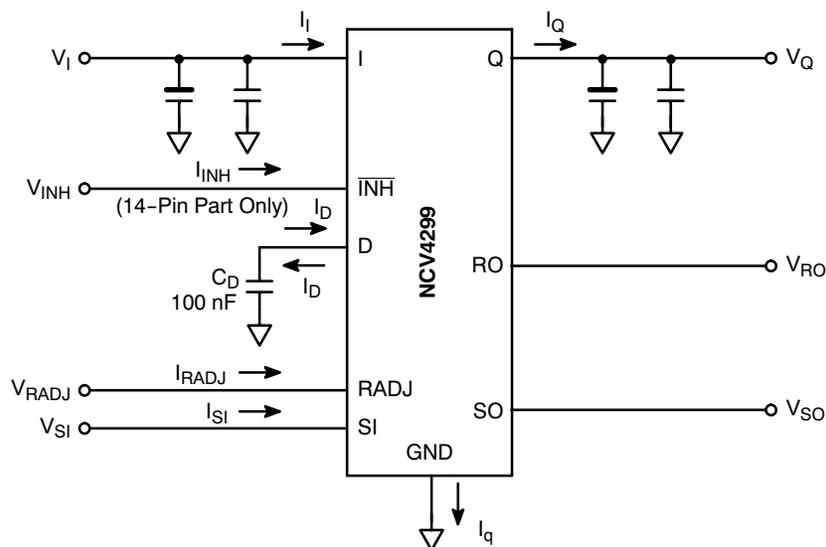
**Figure 3. Measurement Circuit**
