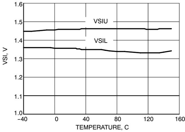
Figure 10. Sense Threshold VSI vs. Temperature  $T_J$
