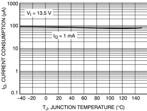
Figure 19. Current Consumption vs. Junction Temperature
