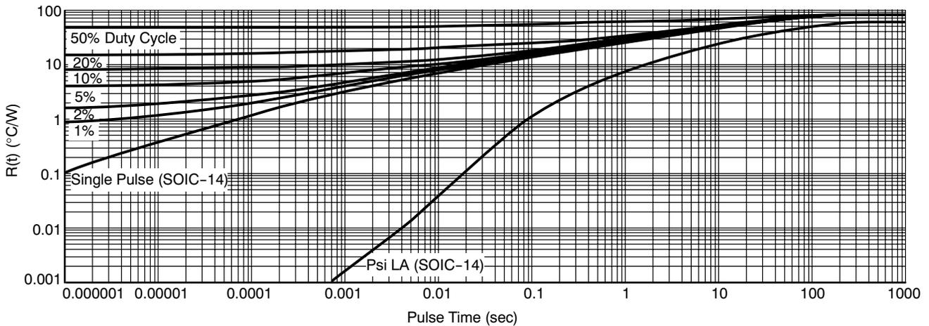
Figure 49. Transient Thermal Response Simulation to a Single Pulse with Duty Cycles Applied (Log-Log)
