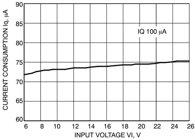
Figure 16. Current Consumption Iq vs. Input Voltage VI
