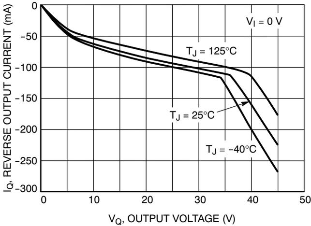
Figure 23. Reverse Output Current vs. Output Voltage
