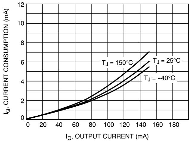
Figure 20. Current Consumption vs. Output Current
