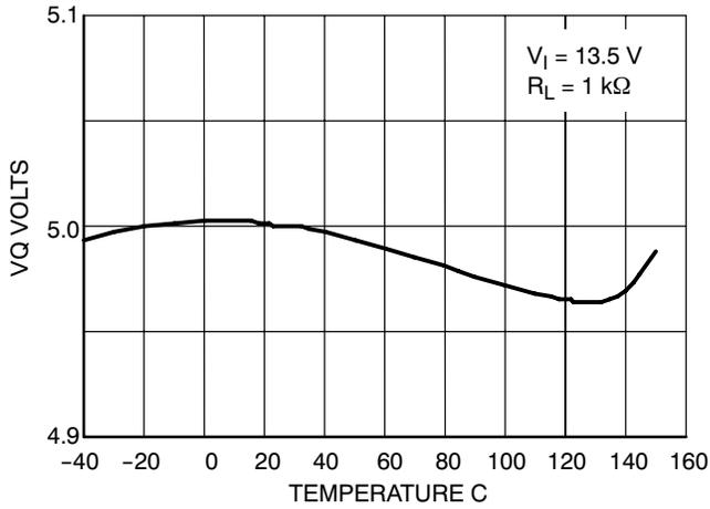
Figure 4. Output Voltage VQ vs. Temperature TJ
