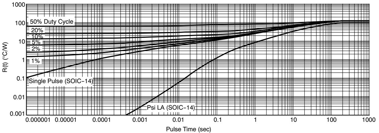
Figure 48. Transient Thermal Response Simulation to a Single Pulse with Duty Cycles Applied (Log-Log)
