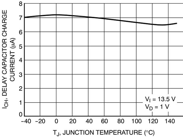
Figure 33. Delay Capacitor Charge Current vs. Junction Temperature
