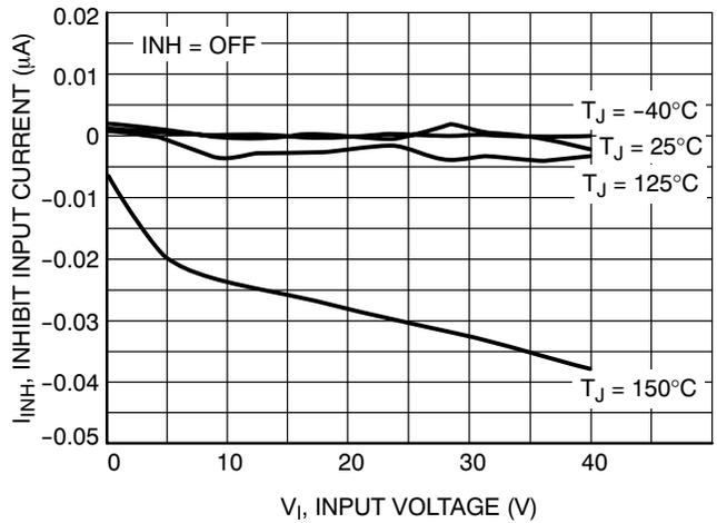
Figure 28. Inhibit Input Current at Input Voltage Extremes
