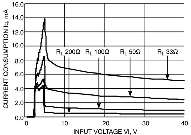
Figure 15. Current Consumption  $I_q$  vs. Input Voltage  $V_I$
