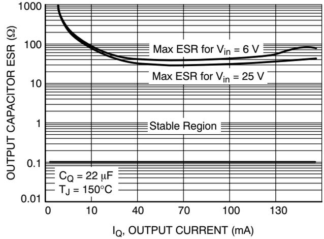
Figure 26. 3.3 V Output Stability with Output Capacitor ESR
