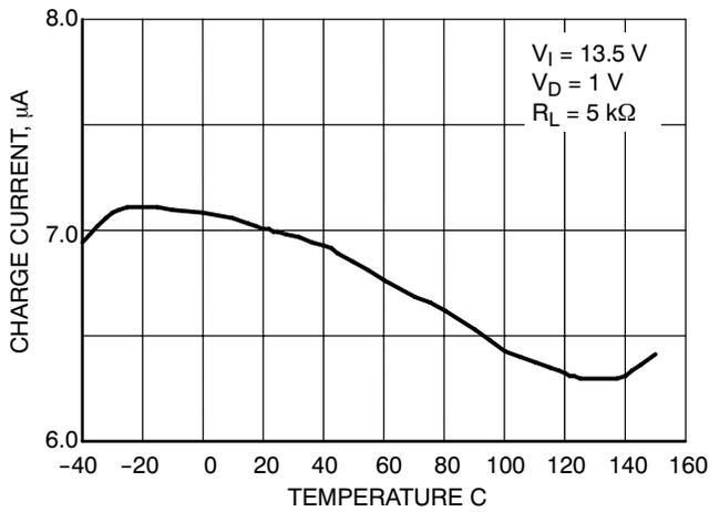
Figure 6. Charge Current Id, c vs. Temperature TJ
