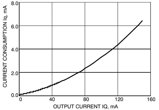
Figure 13. Current Consumption  $I_q$  vs. Output Current  $I_Q$
