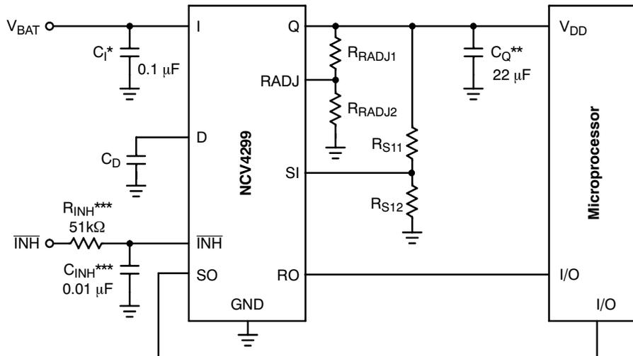
\* $C_I$  required if regulator is located far from the power supply filter.
