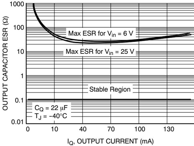
Figure 27. 3.3 V Output Stability with Output Capacitor ESR
