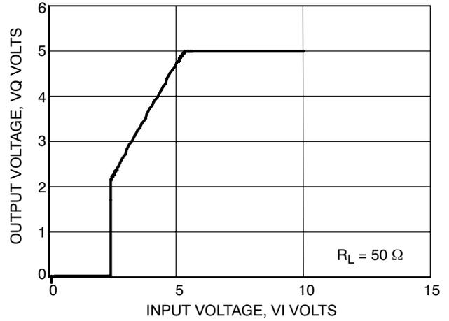
Figure 5. Output Voltage VQ vs. Input Voltage
