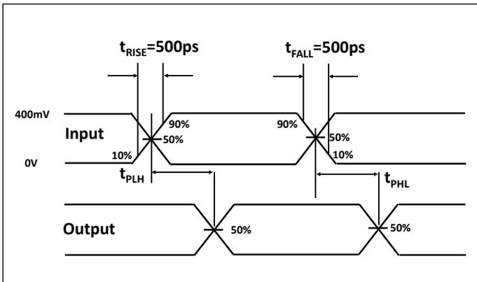
**Fig 3. Skew Test**
