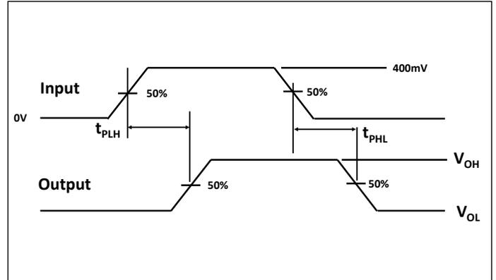
**Fig 2. Propagation Delay**
