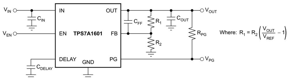
Figure 14. TPS7A1601 Circuit as an Adjustable Regulator Schematic
