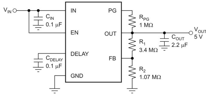
**Figure 15. Adjustable Operation**
