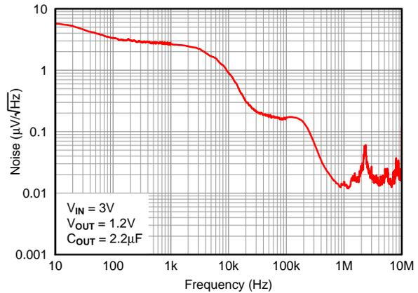
Figure 12. Output Spectral Noise Density
