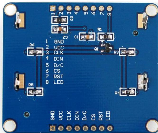
If you want to use the backlight, that can draw up to 80mA (4 white LEDs at 20mA each). The backlight pin is connected to a transistor so you can PWM all 4 LEDs at once from a microcontroller pin.
