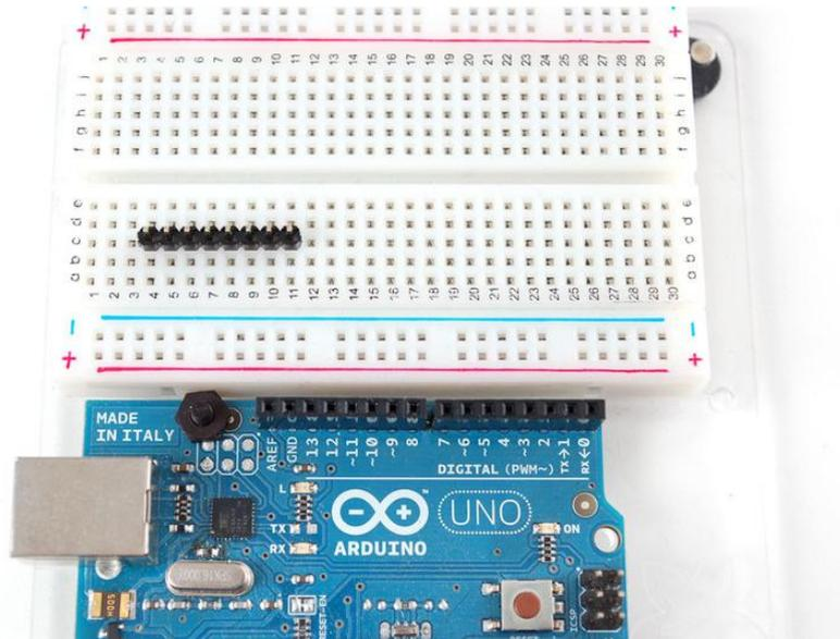
Slide either side of the LCD onto the header, the 'thicker' end is the top.
