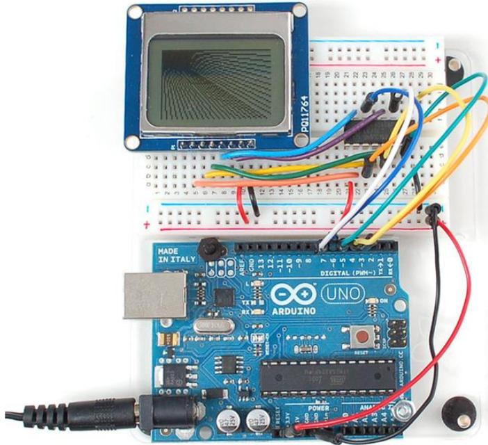
You can save some pins by connecting the CS pin to ground (this means you cant reuse the LCD's pins between screen updates but maybe thats OK. You can also connect the RST pin to the Arduino reset so that it will reset the screen automatically.
