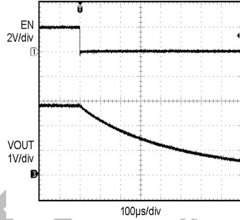
Figure 18. Enable Turn-off (100 μA Load)
