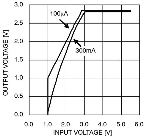
Figure 3. Dropout Characteristics
