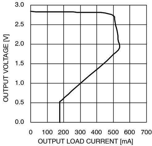
Figure 9. Output Voltage vs. Load Current
