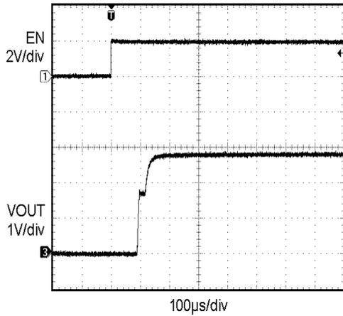
Figure 17. Enable Turn-on (100 μA Load)
