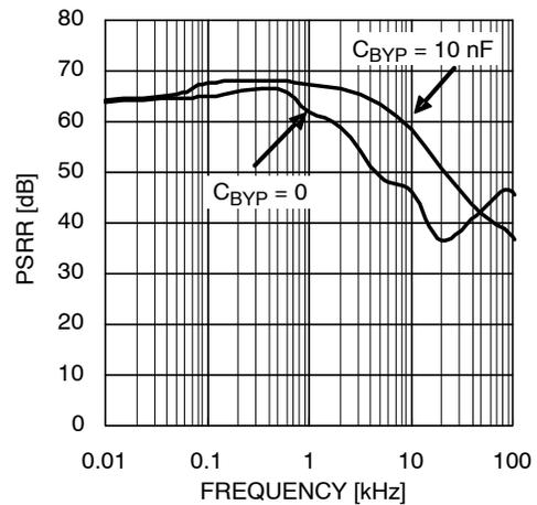
Figure 14. PSRR vs. Frequency (10 mA Load)
