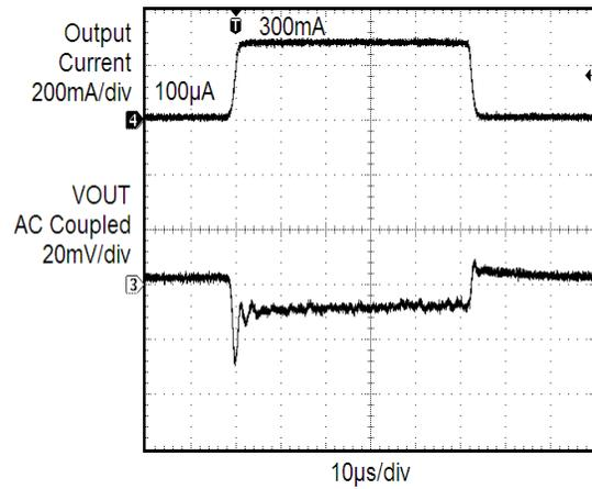
Figure 22. Load Transient Response (0.1 mA to 300 mA)
