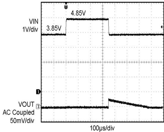
Figure 21. Line Transient Response (3.85 V to 4.85 V)
