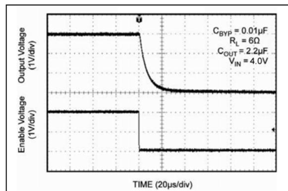
**FIGURE 2-23:** Shutdown Delay (3.0V Fixed Output Version).
