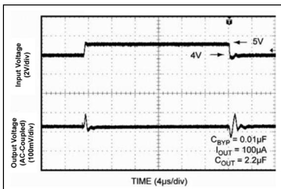
**FIGURE 2-20:** Line Transient Response (3.0V Fixed Output Version).
