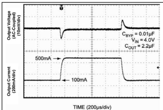
**FIGURE 2-21:** Load Transient Response (3.0V Fixed Output Version).
