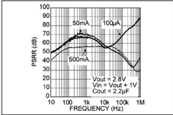
**FIGURE 2-1:** PSRR (Bypass Pin Capacitor = 0.1  $\mu\text{F}$ ).
