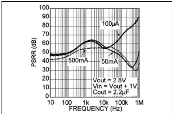
**FIGURE 2-2:** PSRR (Bypass Pin Capacitor = 0.01  $\mu\text{F}$ ).
