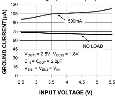
**Ground Current vs. Output Current**
