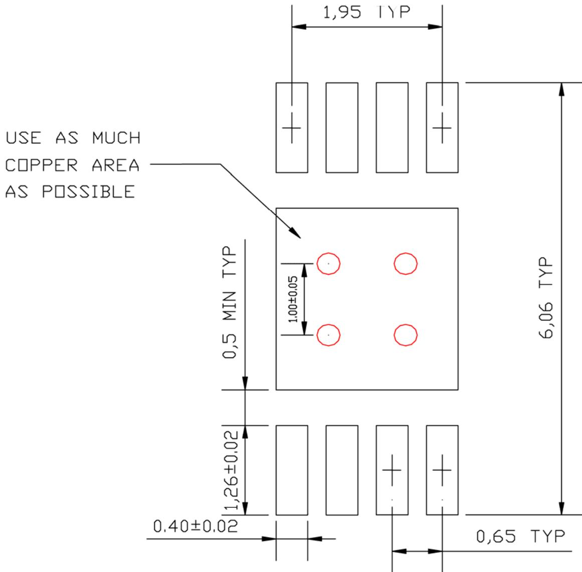
**Red circle** indicates Thermal Via. Size should be .300 – .350mm in diameter, 1/00mm pitch, and it should be connected to GND plane for maximum thermal performance.
