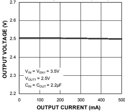
**Output Voltage vs. Output Current (V<sub>OUT2</sub>)**
