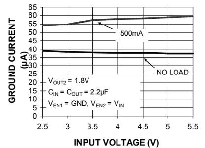
**Ground Current vs. Input Voltage (Dual Output)**
