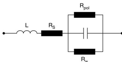
The ESR comprises the polarization losses of the dielectric material (R<sub>pol</sub>), the losses caused by the resistance of the leads, termination and electrodes (R<sub>s</sub>) and the insulation resistance (R<sub>is</sub>).
