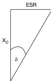
The tan δ reflects the polarization losses of the dielectric film and the losses caused by the contact resistance (terminals - scooping - electrodes) of the capacitor. Parallel losses can, due to the high insulation resistance of film capacitors, be neglected. The tan δ is temperature and frequency dependent.
