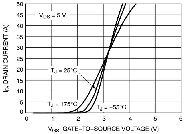
Figure 2. Transfer Characteristics
