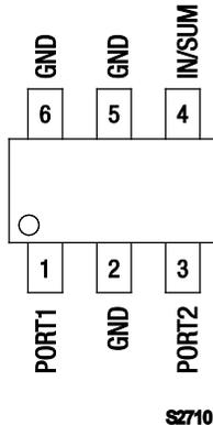
**Figure 2. PD18-73/PD18-73LF Pinout – 6-Pin SOT-6 (Top View)**
