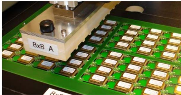
Radiocrafts ATS – Automatic Test Station – module boards
