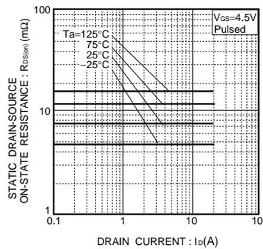
Fig.7 Static Drain-Source On-State Resistance vs. Drain Current (2)
