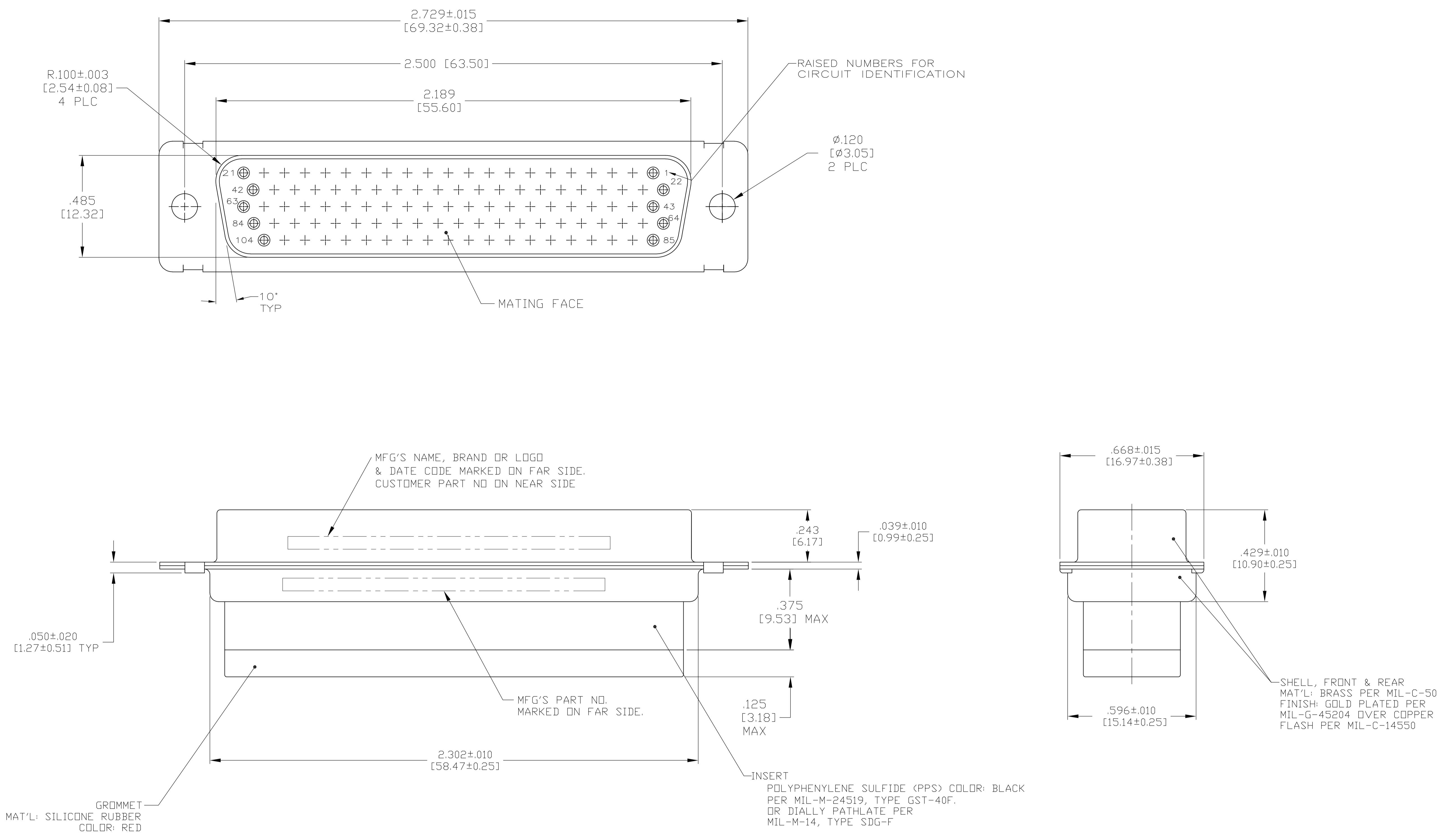
1. THIS RECEPTACLE WILL MATE WITH ANY SIZE 6, 104 POSN. PLUG IN AMPLIMITE SERIES.
