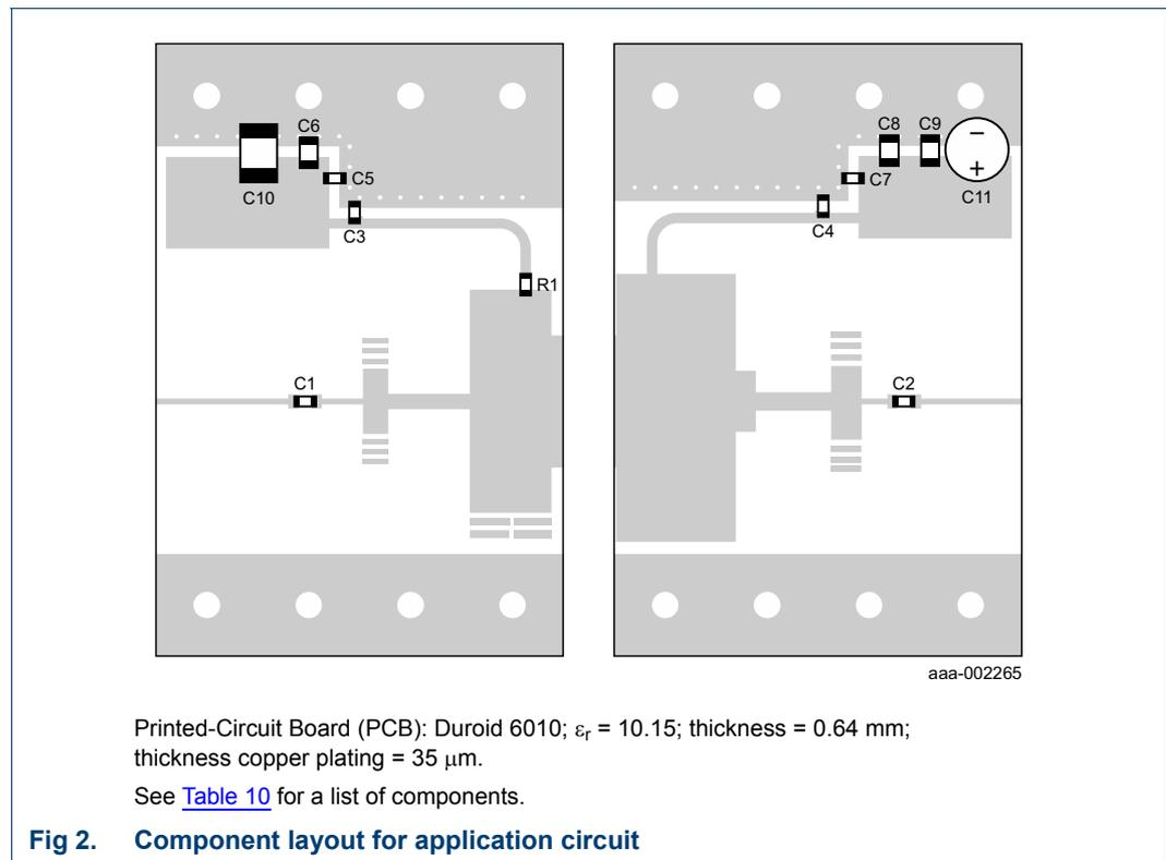
Printed-Circuit Board (PCB): Duroid 6010;  $\epsilon_r = 10.15$ ; thickness = 0.64 mm;
