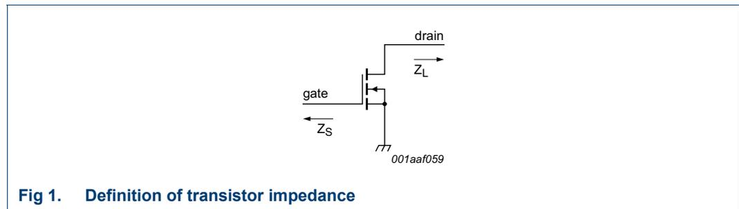
**Fig 1. Definition of transistor impedance**
