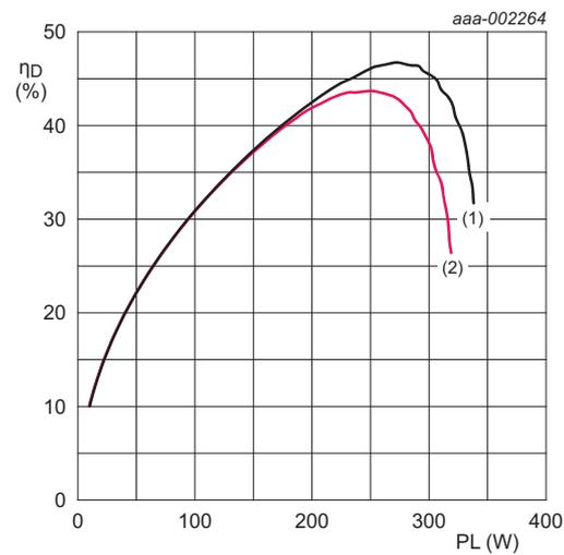
$f = 1300\text{ MHz}; t_p = 100\ \mu\text{s}; \delta = 10\%$ .
