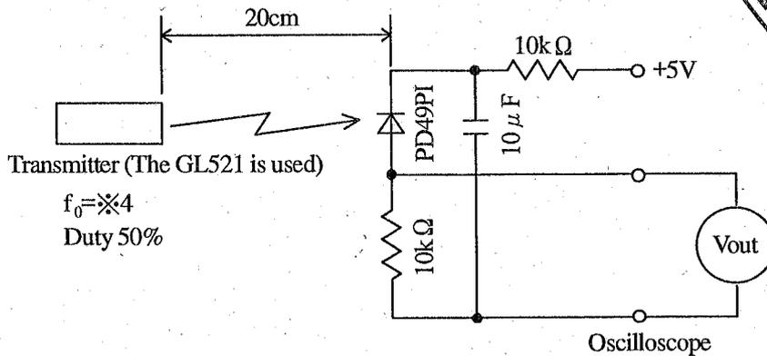
In the figure above, the transmitter shall be set as the output Vout (p-p) will be 40mV.
