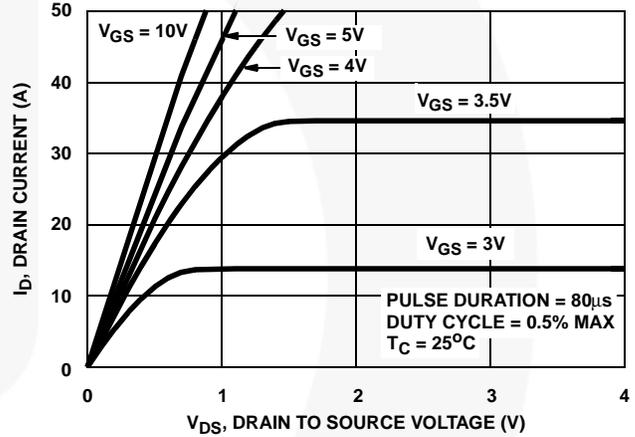
FIGURE 8. SATURATION CHARACTERISTICS
