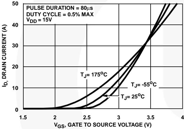
FIGURE 7. TRANSFER CHARACTERISTICS
