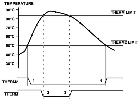
Figure 9. Operation of the  $\overline{\text{THERM}}$  and  $\overline{\text{THERM2}}$  Interrupts
