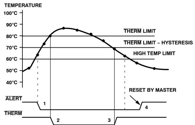
**Figure 8. Operation of the  $\overline{\text{ALERT}}$  and  $\overline{\text{THERM}}$  Interrupts**
