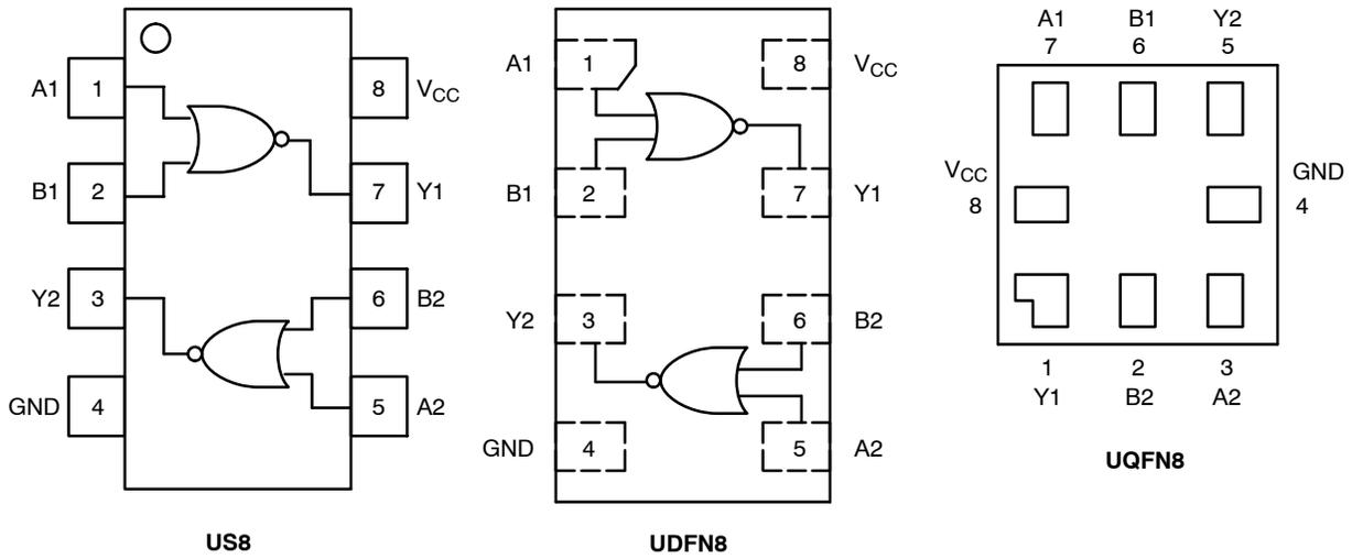
Figure 2. Pinout
