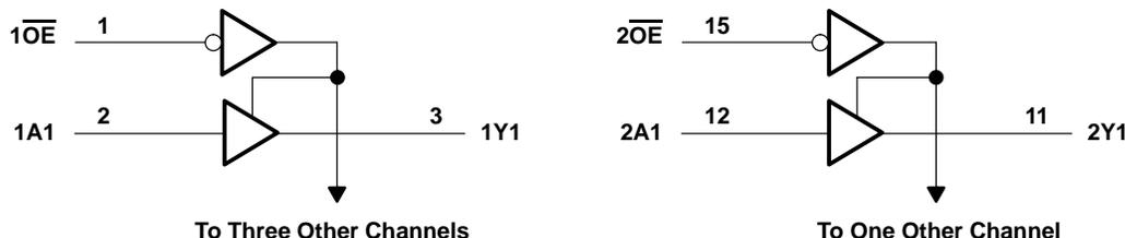
Pin numbers shown are for the D, DB, DGV, J, N, PW, and W packages.
