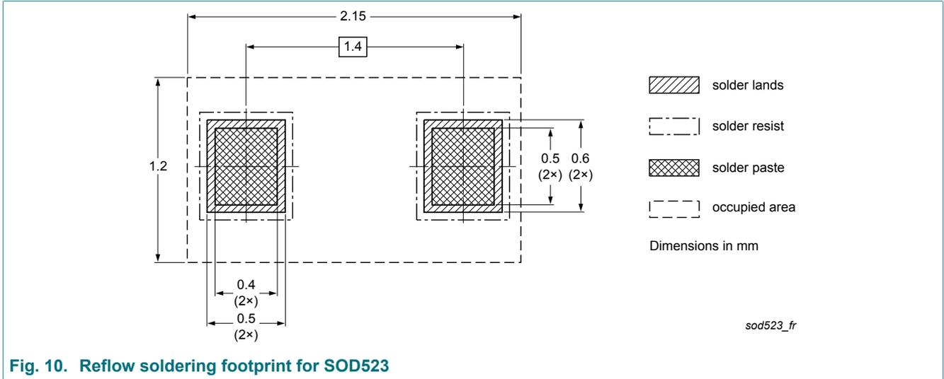
Fig. 10. Reflow soldering footprint for SOD523
