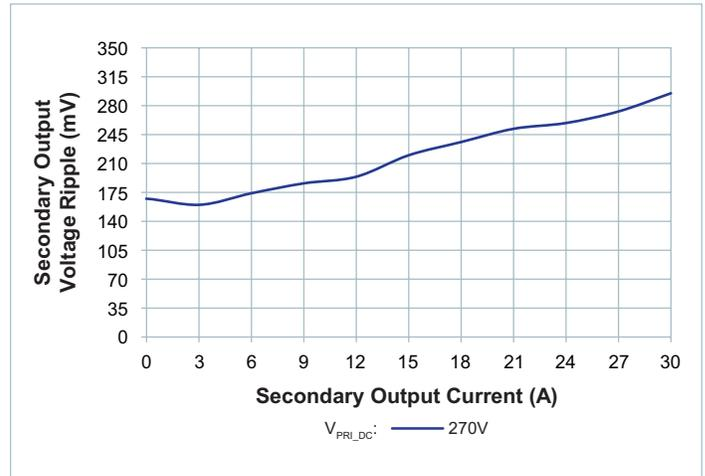
Figure 13 —  $V_{SEC\_OUT\_PP}$  vs.  $I_{SEC\_DC}$ ; no external  $C_{SEC\_OUT\_EXT}$ .
