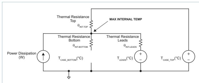
Figure 23 — Top case and leads thermal model
