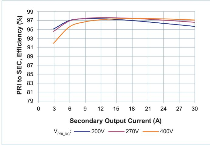
Figure 10 — Efficiency at  $T_{CASE} = 100^{\circ}C$
