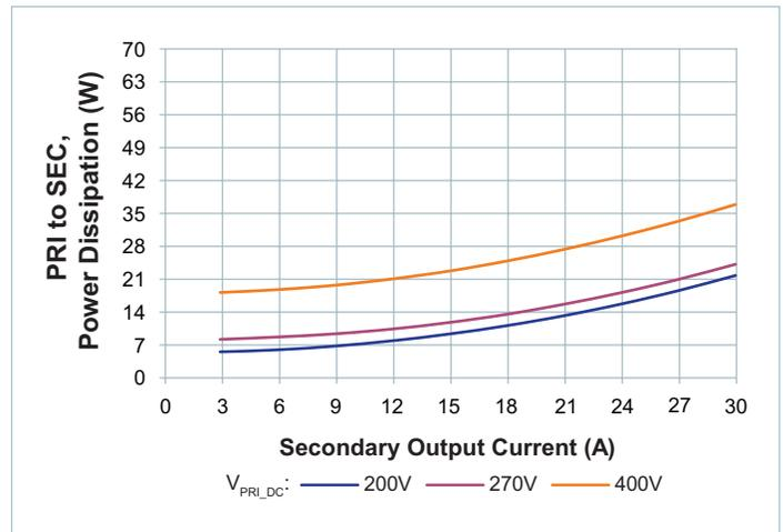
Figure 7 — Power dissipation at  $T_{CASE} = -55^{\circ}C$
