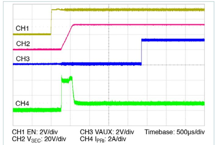
Figure 18 — Start up from application of  $EN$  with pre-applied
