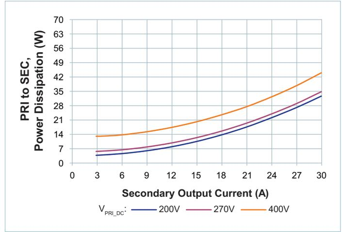
Figure 11 — Power dissipation at  $T_{CASE} = 100^{\circ}C$
