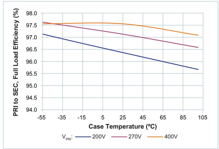
Figure 5 — Full-load efficiency vs. temperature;  $V_{PRI\_DC}$
