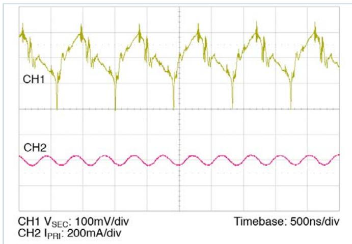
Figure 14 — Full-load secondary voltage and primary current ripple,  $10\mu F C_{PRI\_IN\_EXT}$ ; no external  $C_{SEC\_OUT\_EXT}$ .
