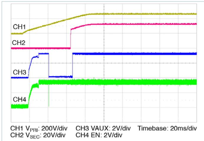
Figure 17 — Start up from application of  $V_{PRI\_DC} = 270V$ ,
