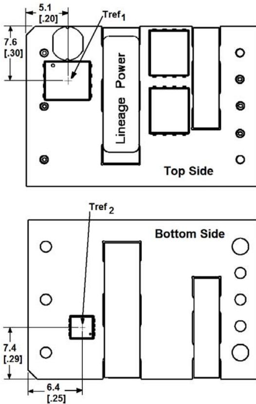
Figure 19. Tref<sub>x</sub> Temperature Measurement Location.
