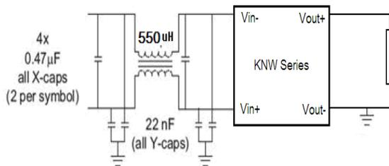
Figure 20. Single stage filter used for test results.
