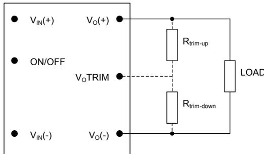
**Figure 18. Circuit Configuration to Trim Output Voltage.**
