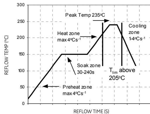
Figure 23. Reflow Profile for Tin/Lead (Sn/Pb) process
