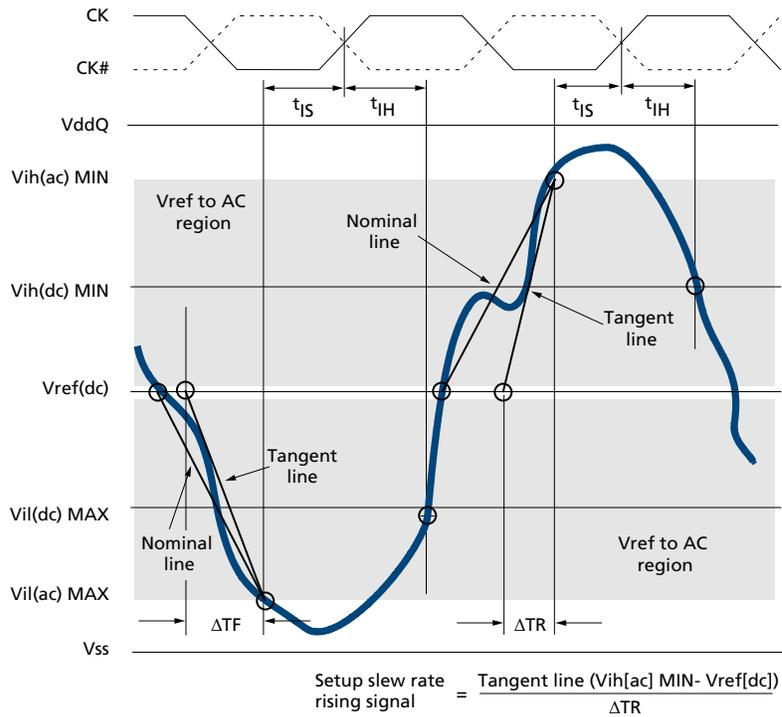
Figure 24: Nominal Slew Rate for  $t_{IH}$
