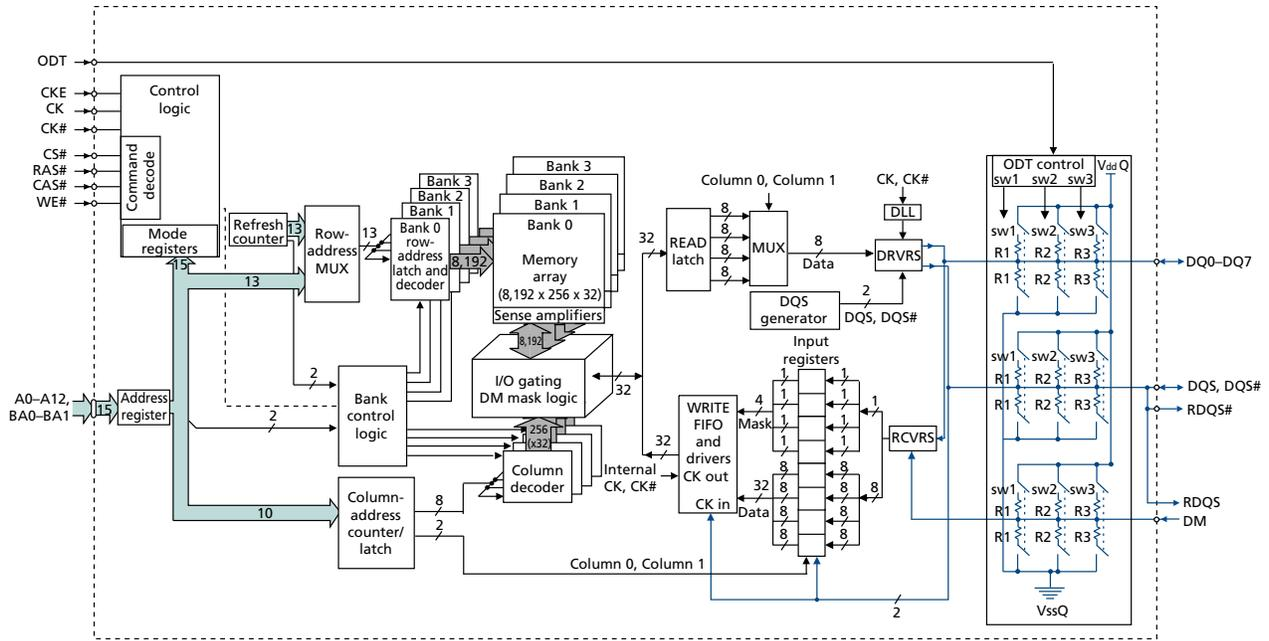
Figure 5: 16 Meg x 16 Functional Block Diagram
