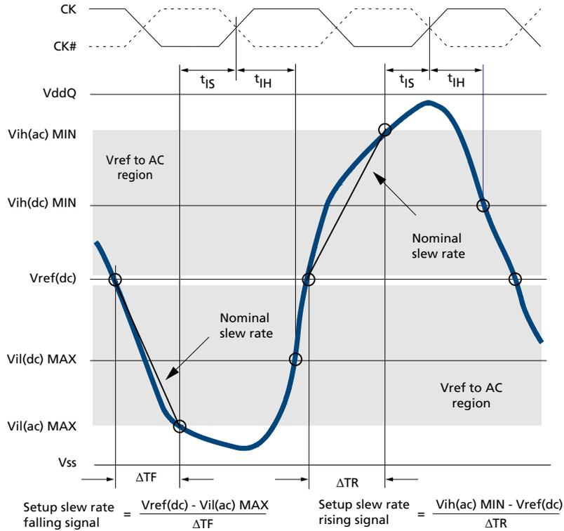
Figure 23: Tangent Line for  $t_{1S}$
