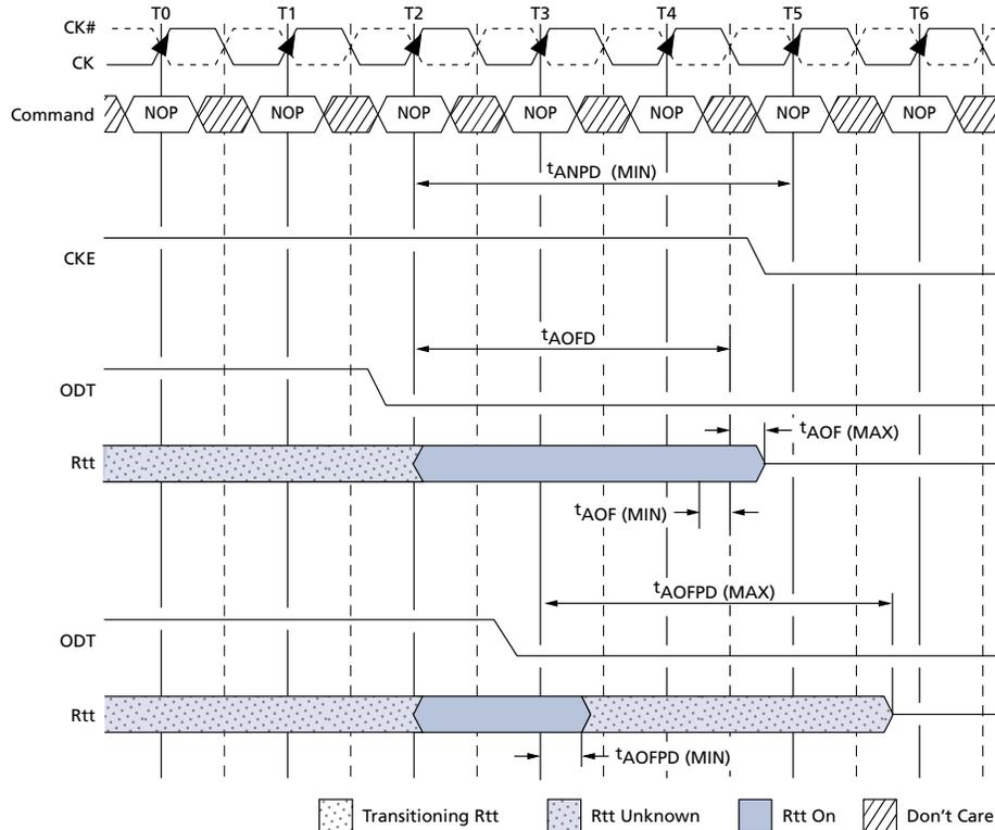
Figure 84: ODT Turn-On Timing When Entering Power-Down Mode
