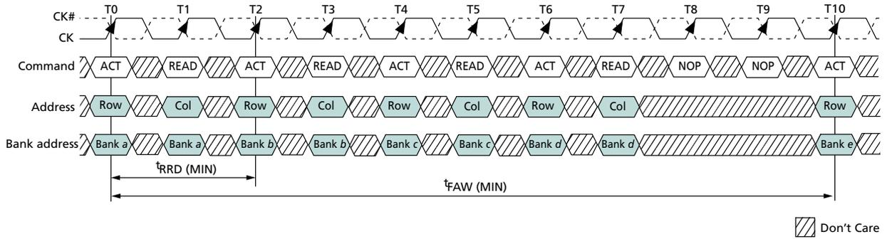
Note: 1. DDR2-533 (-37E, x4 or x8),  $t_{CK} = 3.75ns$ ,  $BL = 4$ ,  $AL = 3$ ,  $CL = 4$ ,  $t_{RRD} (MIN) = 7.5ns$ ,  $t_{FAW} (MIN) = 37.5ns$ .
