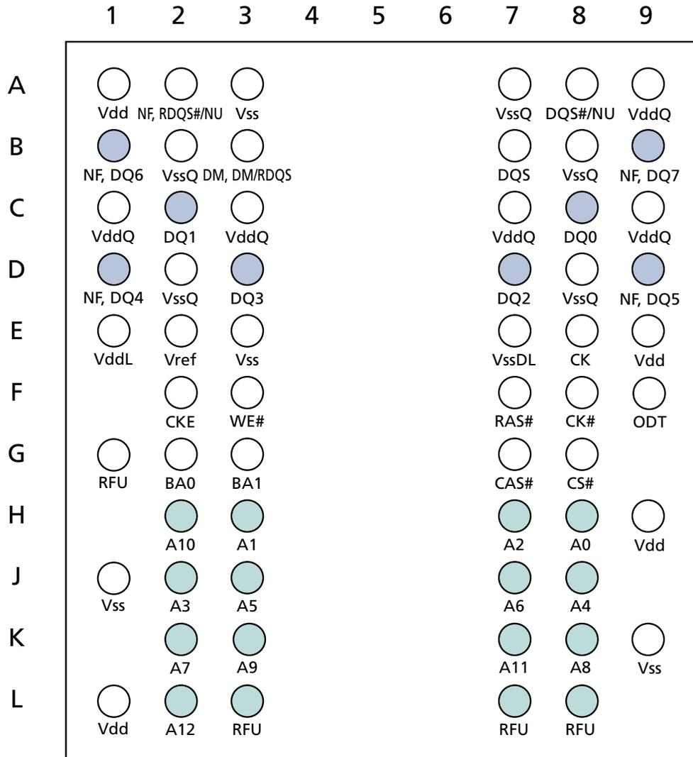
**Figure 7: 84-Ball FBGA – x16 Ball Assignments (Top View)**
