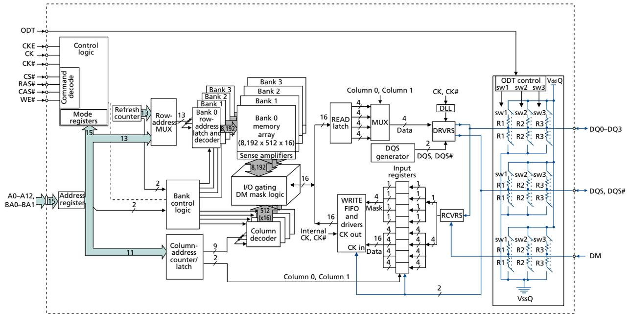
Figure 4: 32 Meg x 8 Functional Block Diagram
