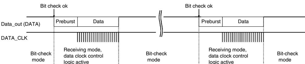
Figure 6-22. Occurrence of a Pulse at the End of the Data Stream
