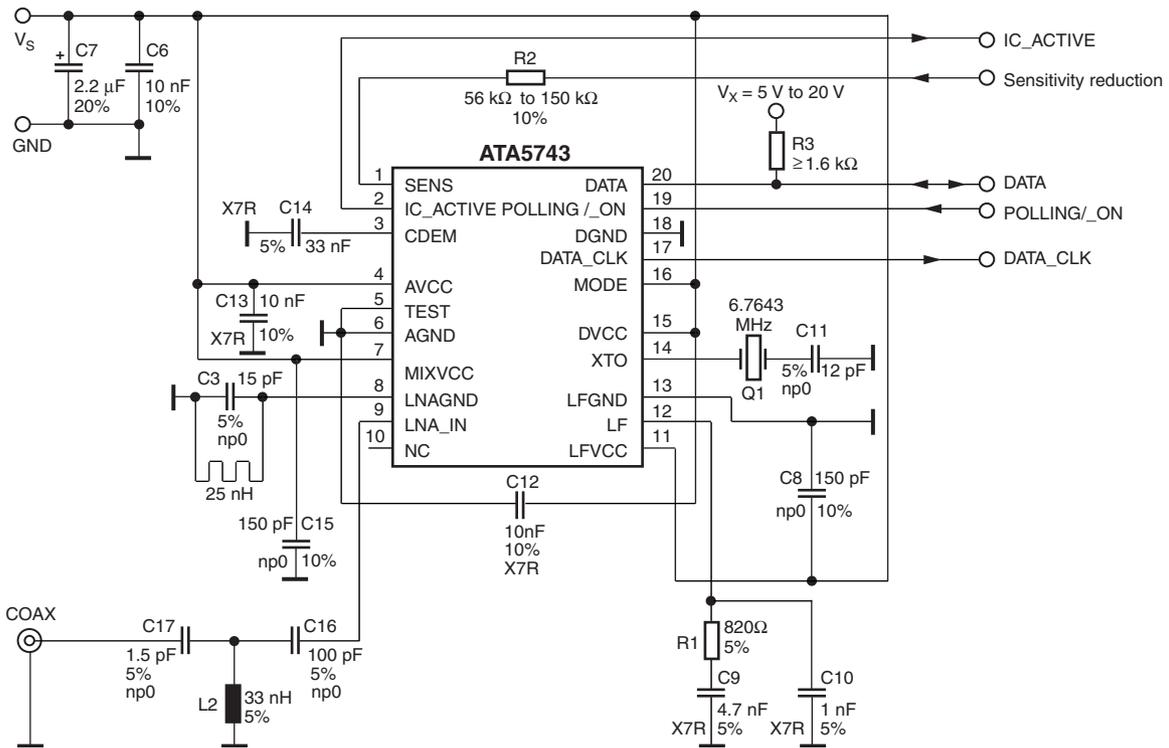
**Figure 6-28.** Application Circuit:  $f_{RF} = 315$  MHz without SAW Filter
