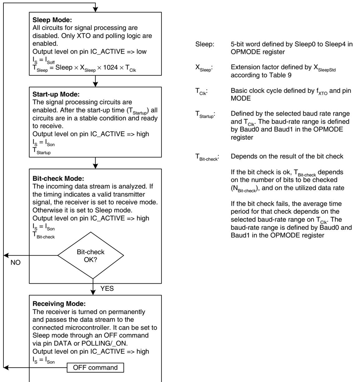
**Figure 6-3.** Timing Diagram for Complete Successful Bit Check
