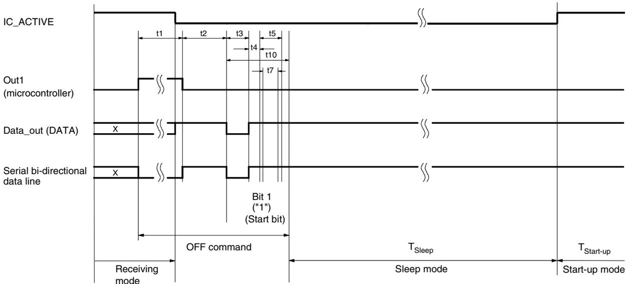
**Figure 6-12.** Timing Diagram of the OFF command via Pin POLLING/\_ON
