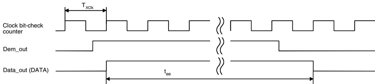
**Figure 6-9.** Debouncing of the Demodulator Output
