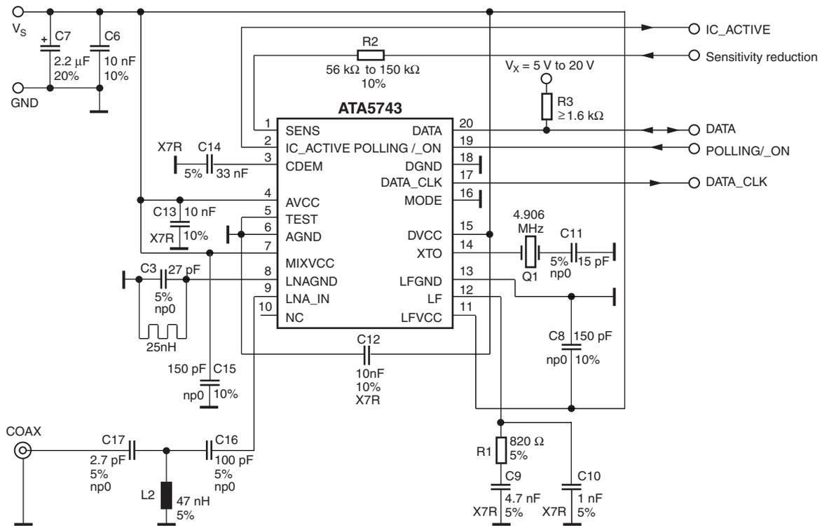
**Figure 6-29.** Application Circuit:  $f_{RF} = 433.92$  MHz with SAW Filter
