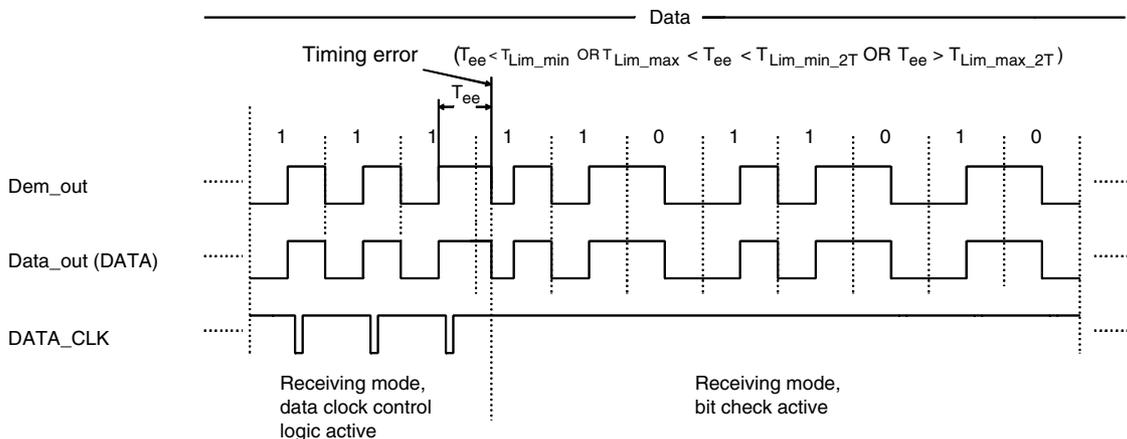
Figure 6-16. Data Clock Disappears Because of a Logical Error
