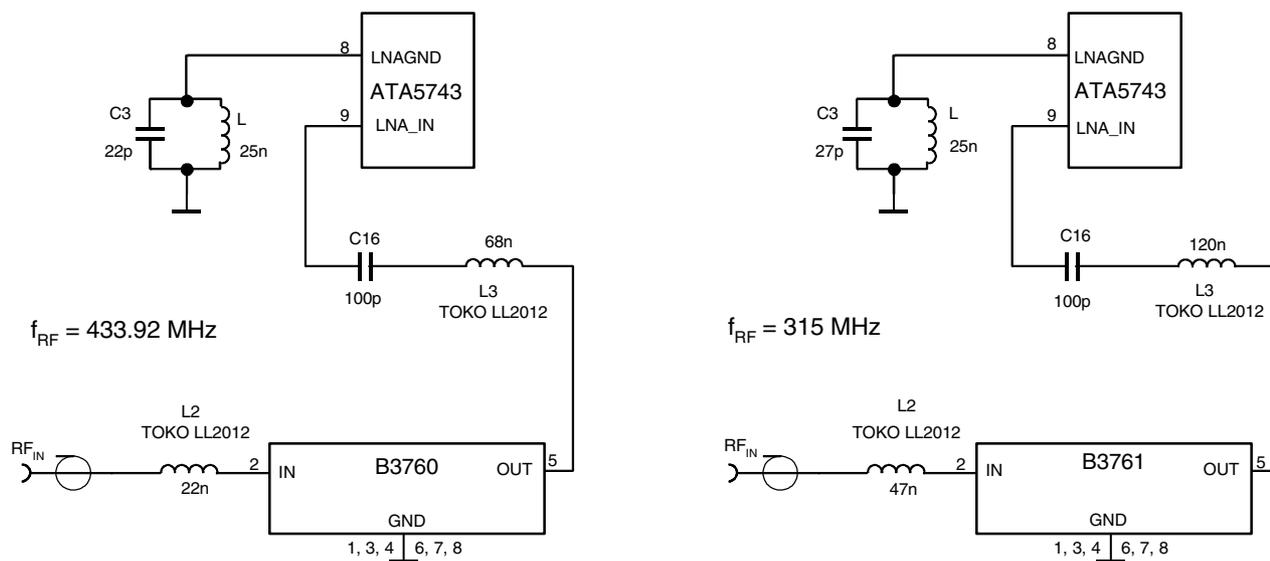
Figure 4-3. Input Matching Network without SAW Filter
