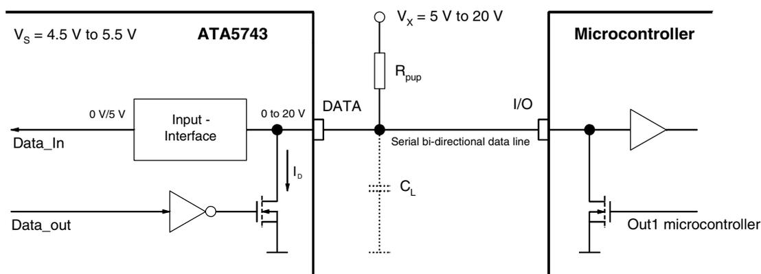
The configuration registers are programmed serially via the bi-directional data line as demonstrated in [Figure 6-25 on page 28](#) and [Figure 6-26](#).
