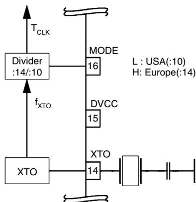
Pin MODE can now be set in accordance with the desired clock cycle  $T_{CLK}$ , which controls the following application relevant parameters:
