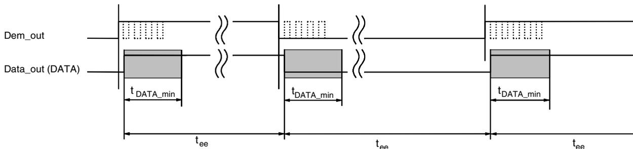
**Figure 6-10.** Steady L State Limited DATA Output Pattern After Transmission
