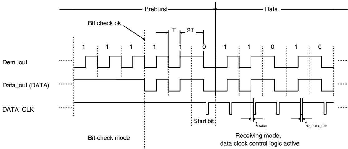
**Figure 6-15.** Data Clock Disappears Because of a Timing Error
