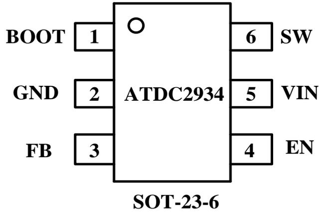
Figure 3. Pin Configuration
