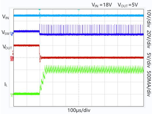
Figure 11. Short-Circuit Entry
