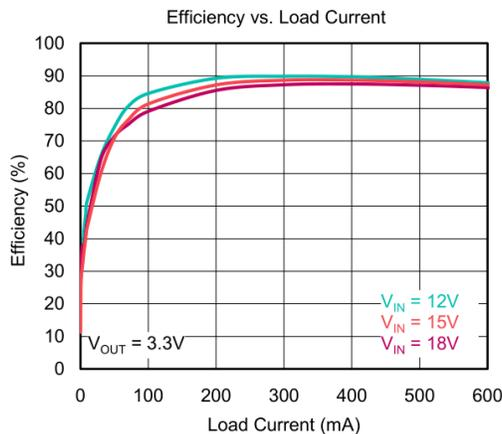
Figure 18. Efficiency vs. Load Current @  $V_{OUT}=3.3\text{V}$
