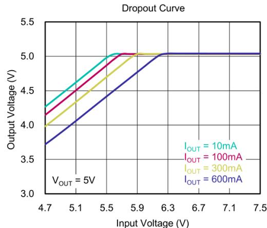
Figure 21. Dropout Curve
