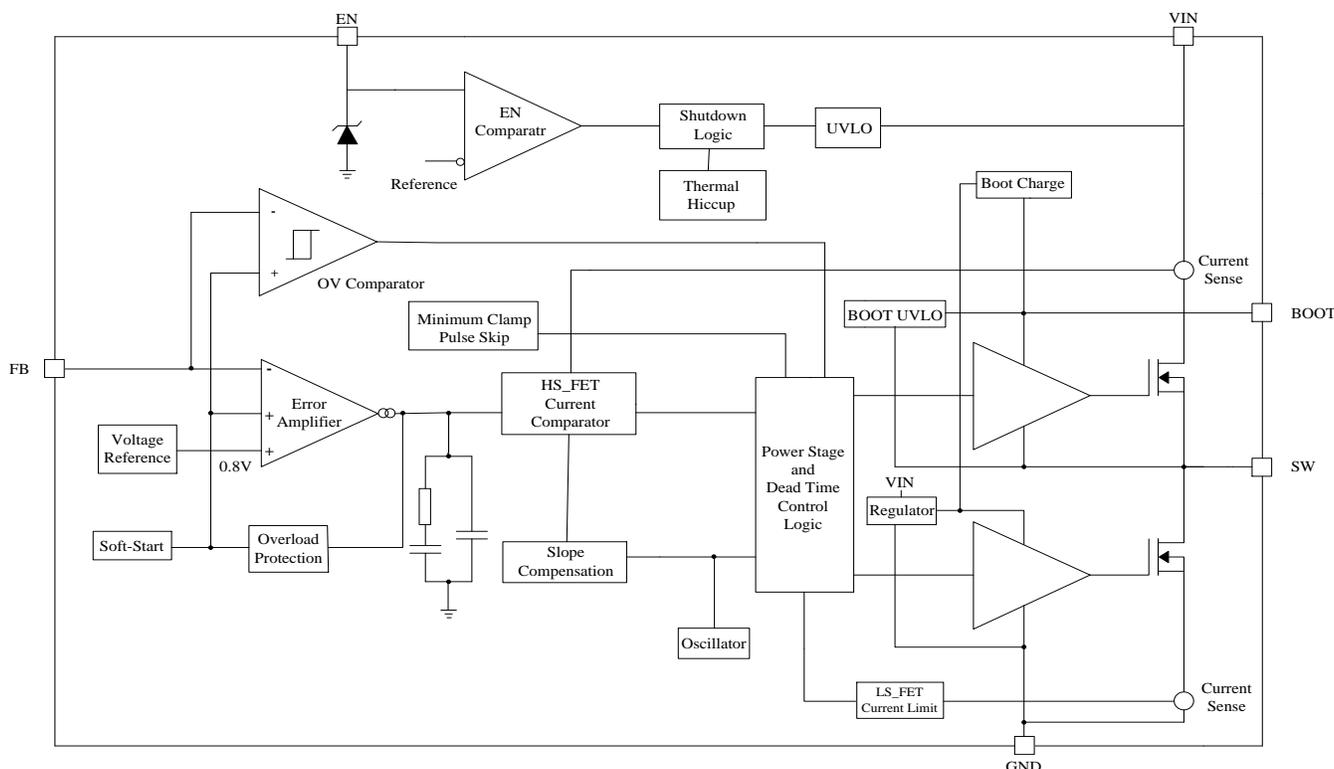
Figure 22. Block Diagram
