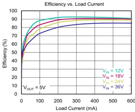
Figure 17. Efficiency vs. Load Current @  $V_{OUT}=5\text{V}$
