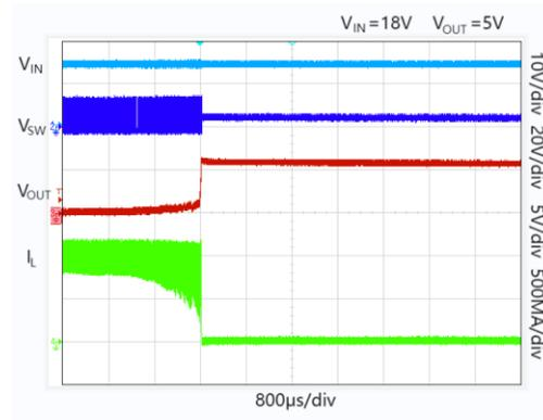
Figure 12. Short-Circuit Recovery
