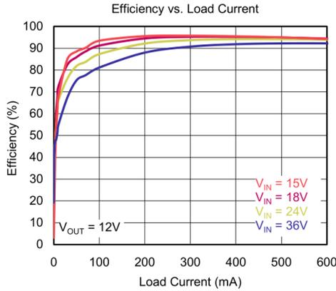
Figure 16. Efficiency vs. Load Current @  $V_{OUT}=12\text{V}$
