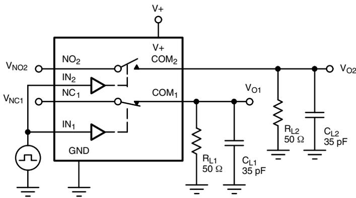
$C_L$  (includes fixture and stray capacitance)
