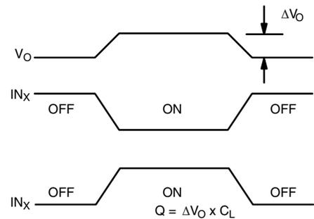
**Figure 3. Charge Injection**
