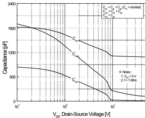
Figure 5. Capacitance Characteristics
