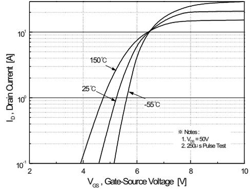
Figure 2. Transfer Characteristics
