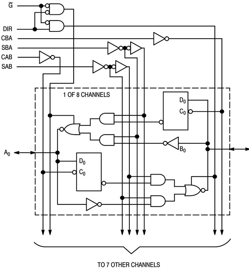
NOTE: This diagram is provided only for the understanding of logic operations and should not be used to estimate propagation delays.
