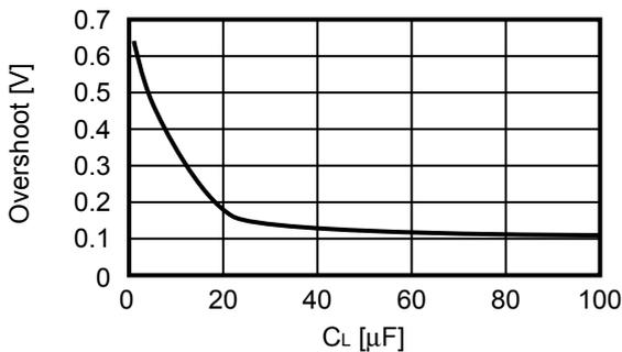
V<sub>IN</sub> = 12.0 V → 7.0 V, t<sub>r</sub> = 5.0 μs, C<sub>IN</sub> = 0.1 μF, I<sub>OUT</sub> = 30 mA
