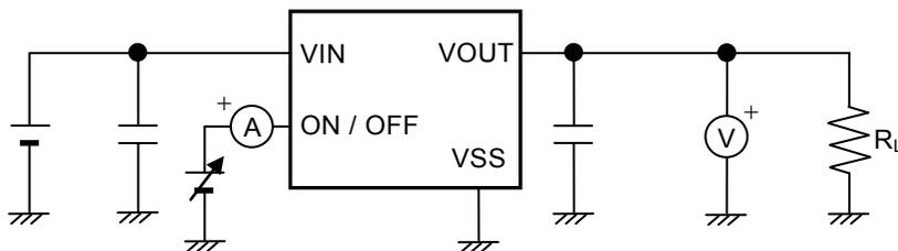
Figure 8 Test Circuit 4
