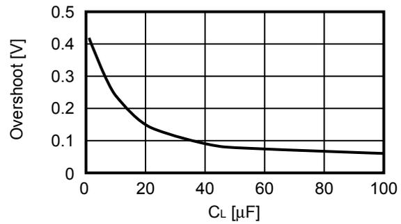
**5. Input transient response characteristics dependent on capacitance (Ta = +25°C)**
