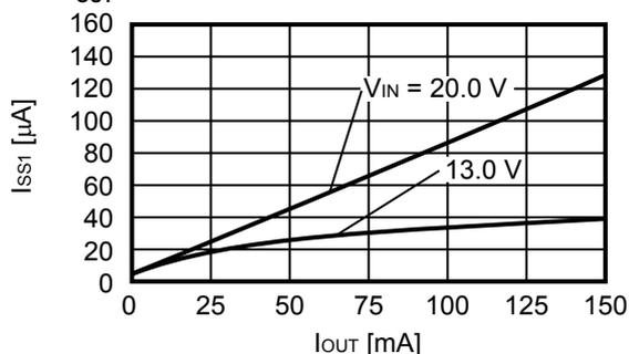
**10. Output current vs. Input voltage\*1**
