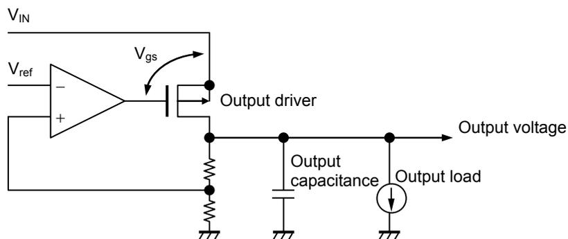
**Figure 13** Circuit Diagram
