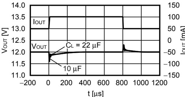
**3. Transient response characteristics of ON / OFF pin (Ta = +25°C)**
