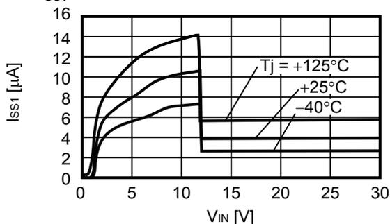
**8. Current consumption during operation vs. Temperature**
