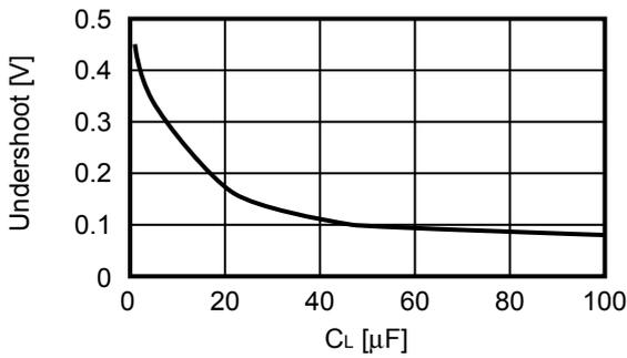
V<sub>IN</sub> = 13.5 V, C<sub>IN</sub> = 0.1 μF, I<sub>OUT</sub> = 100 mA → 50 mA
