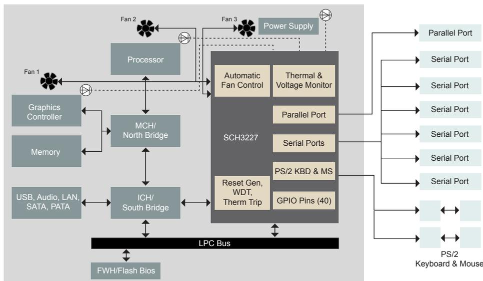
System Controller Hub Application Diagram
