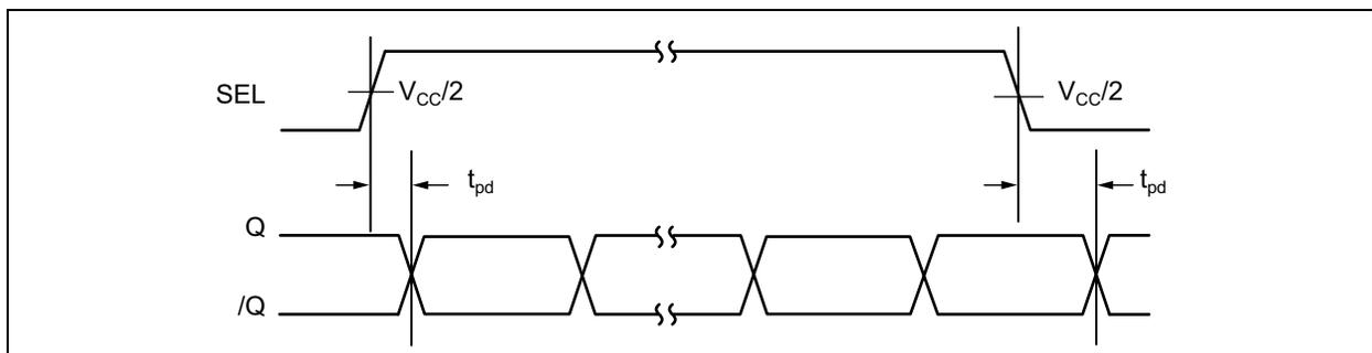
**FIGURE 5-1:** SEL-to-Q Delay.
