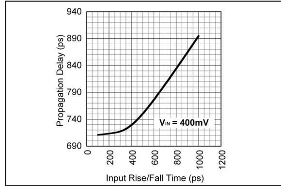
**FIGURE 2-4:** Propagation Delay vs. Input Rise/Fall Time.
