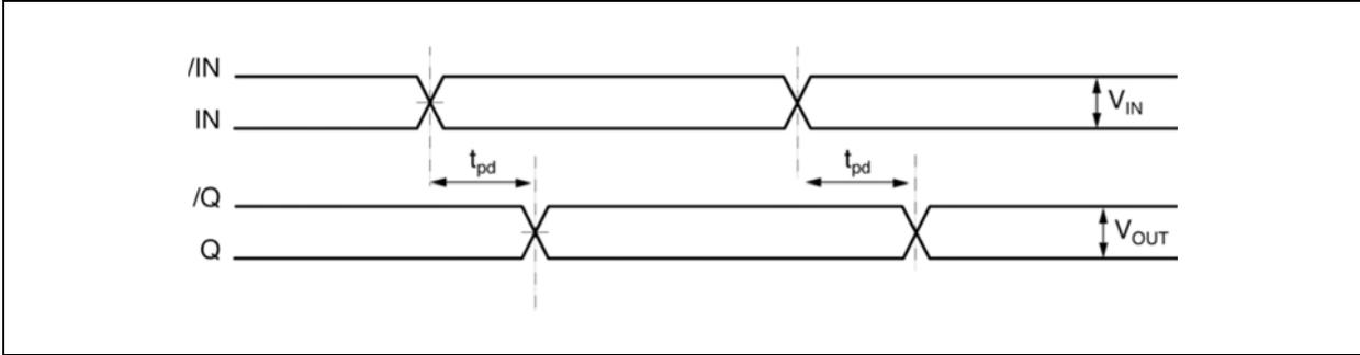
**FIGURE 5-3:** Propagation Delay.
