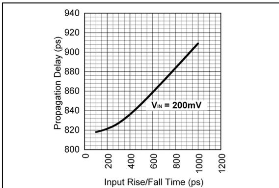
**FIGURE 2-3:** Propagation Delay vs. Input Rise/Fall Time.
