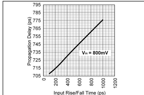
**FIGURE 2-5:** Propagation Delay vs. Input Rise/Fall Time.
