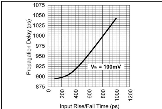
**FIGURE 2-2:** Propagation Delay vs. Input Rise/Fall Time.
