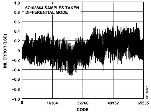
Figure 22. Integral Nonlinearity (Output Data Rate = 1.2 MHz)
