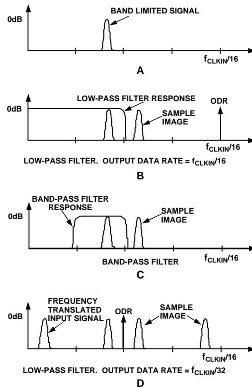
Figure 28. Band-Pass Operation
