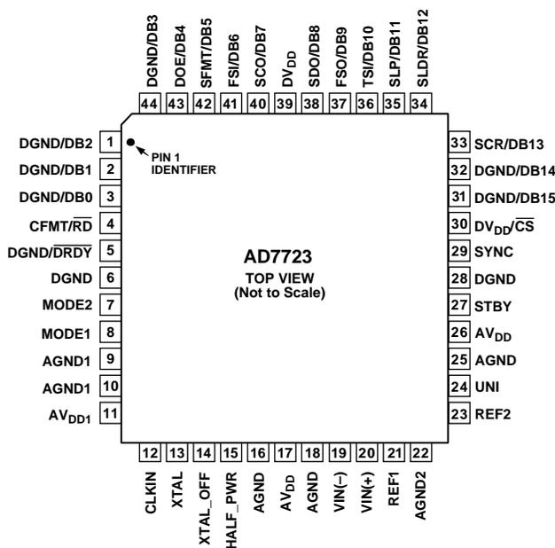
Figure 11. 44-Lead MQFP
