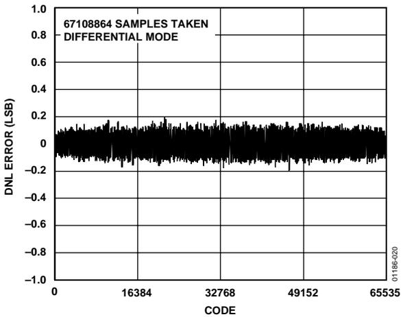
Figure 20. Differential Nonlinearity (Output Data Rate = 1.2 MHz)
