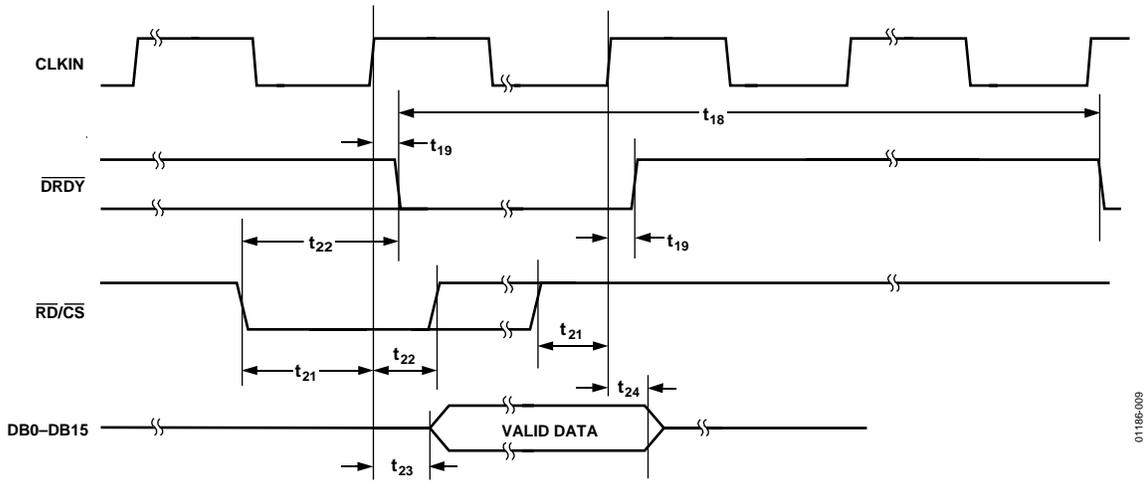
Figure 9. Parallel Mode Read Timing,  $\overline{CS} = \overline{RD}$
