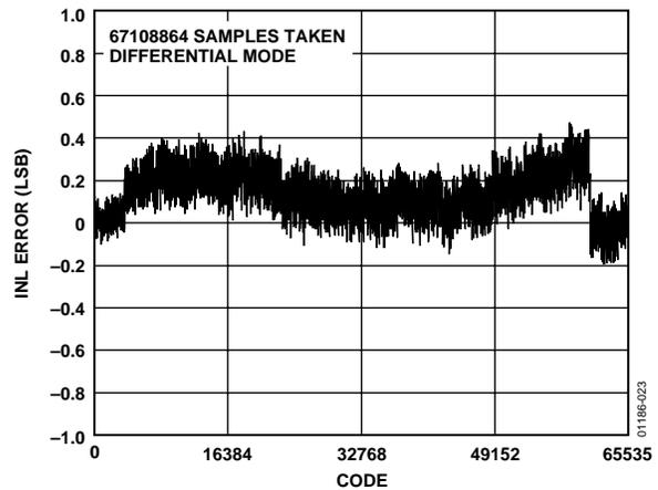
Figure 23. Integral Nonlinearity (Output Data Rate = 600 kHz)
