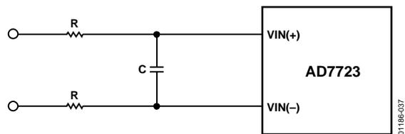
Figure 37. Input RC Network
