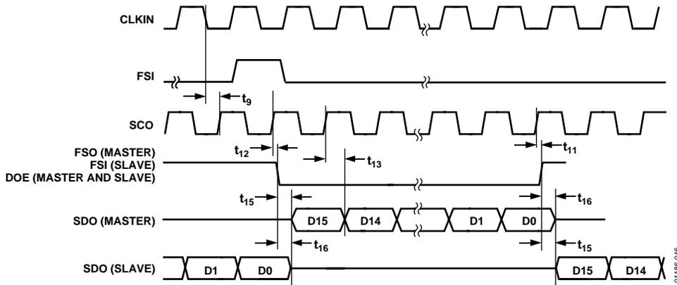
Figure 46. Serial Mode 1 Timing for Two-Channel Multiplexed Operation
