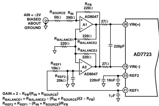
$$GAIN = 2 \times R_{FB} / (R_{IN} + R_{SOURCE})$$
