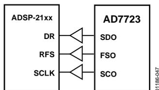
Figure 47. AD7723 to ADSP-21xx Interface
