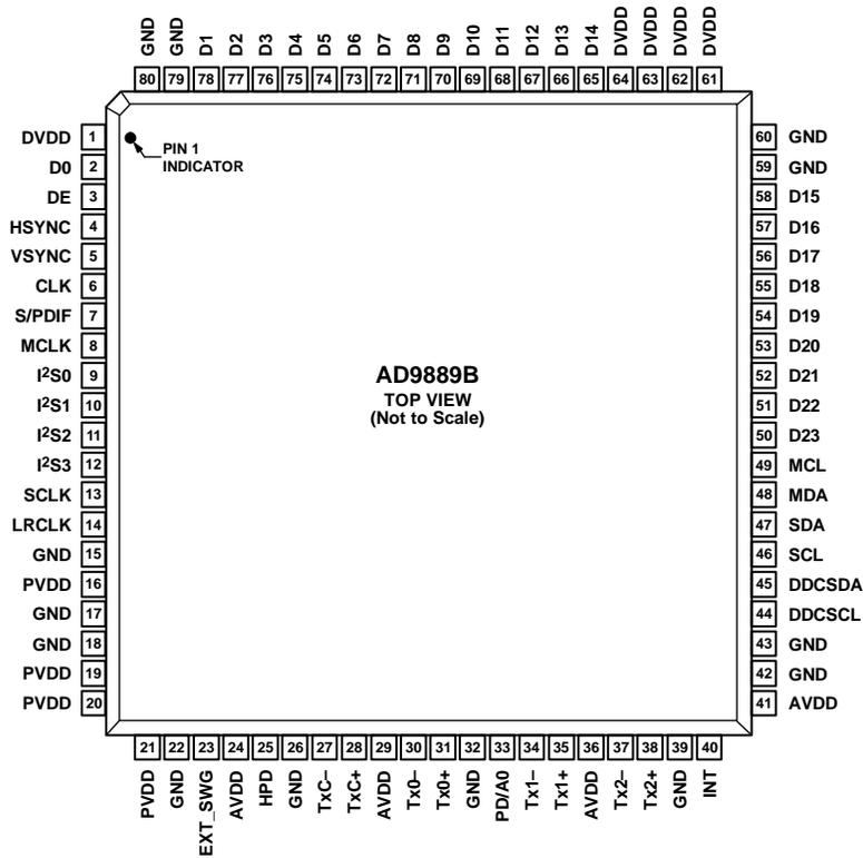
Figure 2. 80-Lead LQFP Pin Configuration (Top View)
