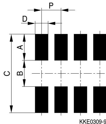
**Recommended dimensions (mm) for reflow soldering**
