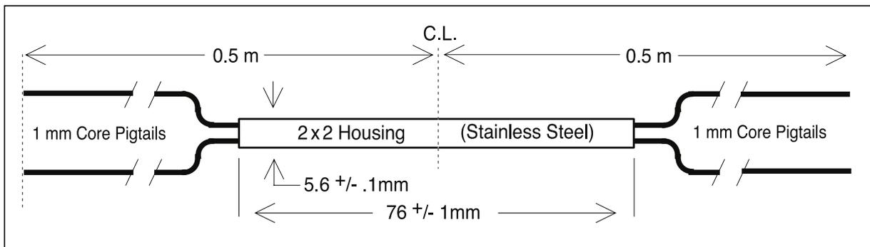
FIGURE 3. Overall Dimensions for 2 × 2 Coupler
