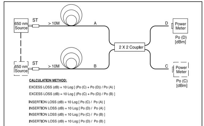
FIGURE 2. Excess & insertion loss measurement - (post-fused)
