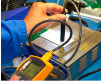
2. Apply localized heat to remove the emitter
