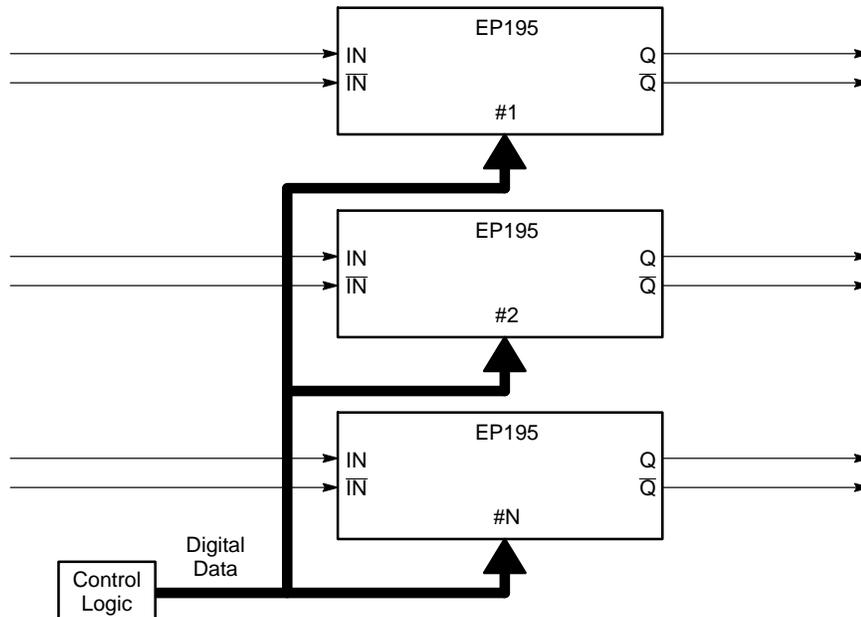
Figure 8. Multiple Channel Deskewing Diagram
