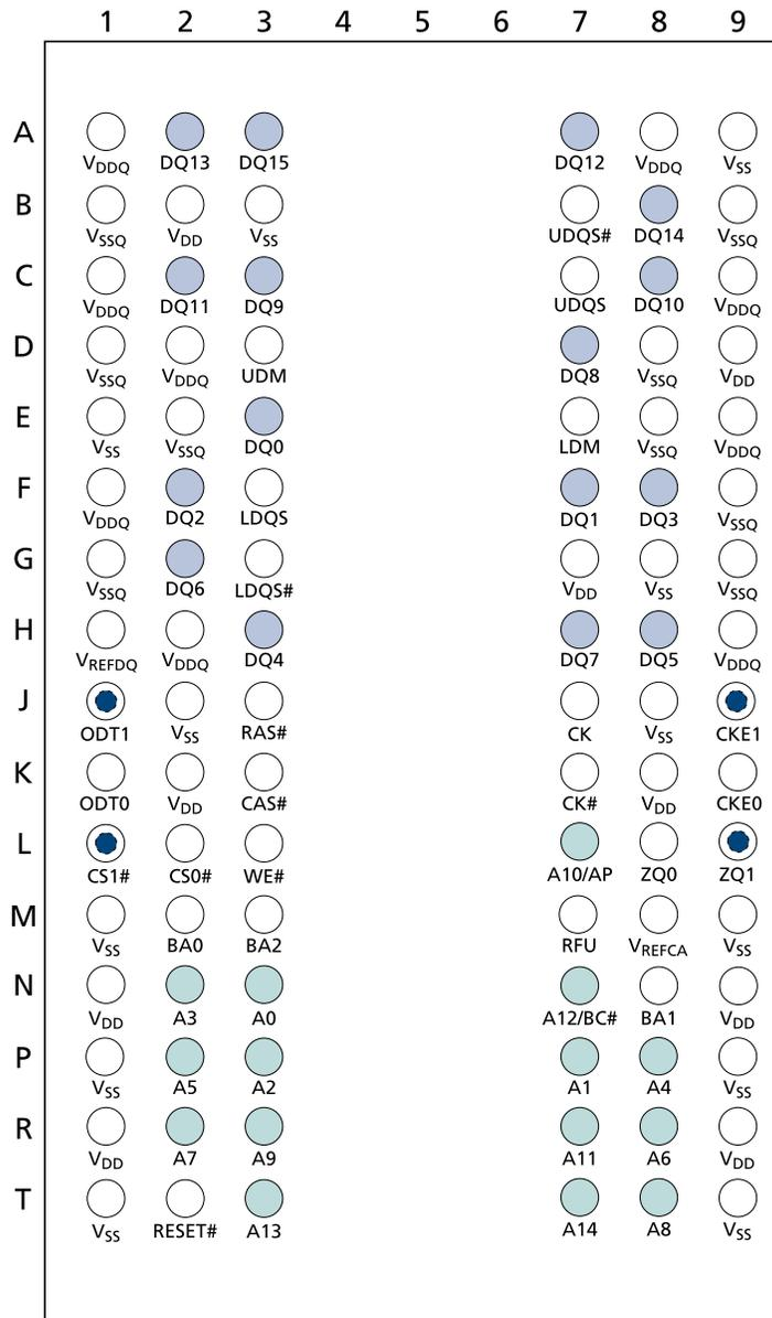
Note: 1. Dark balls (with rings) designate balls that differ from the monolithic versions.
