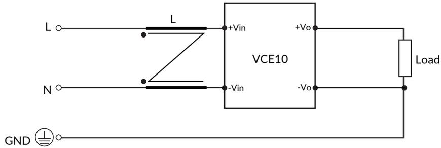
Suggested value - L: 20mH, 500mA common mode choke such as Würth Elektronik 744821120.
