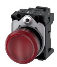
Indicator lights, 22 mm, round, plastic, red, lens, smooth, with holder, LED module, with integrated LED 230 V AC, spring-type terminal, with laser labeling, symbol number according to, ISO 7000 or IEC 60417
