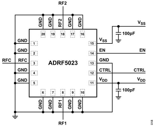
Figure 18. Recommended Schematic
