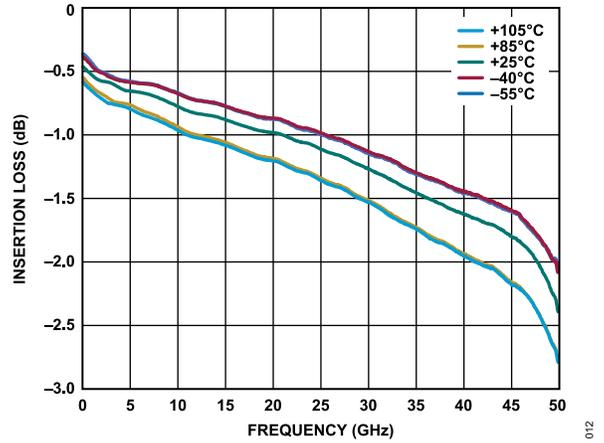
Figure 12. Insertion Loss vs. Frequency over Temperature
