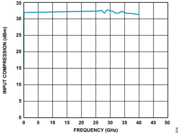
Figure 14. Input 0.1 dB Power Compression vs. Frequency
