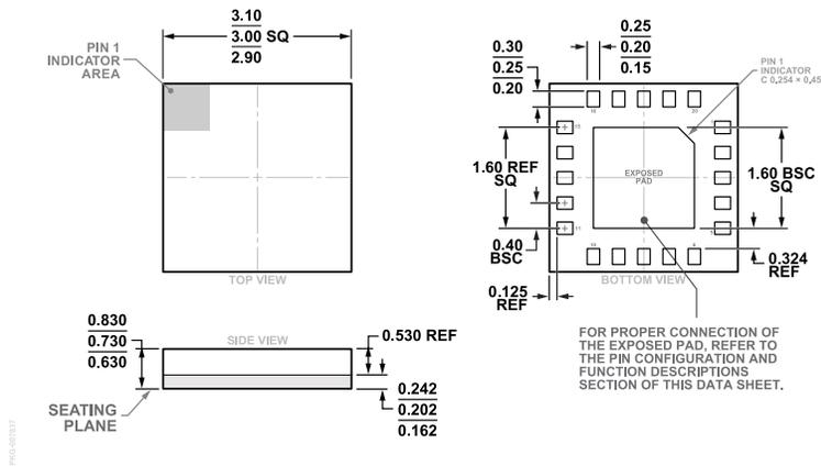
Figure 22. 20-Terminal Land Grid Array [LGA]
