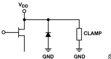
Figure 6. V<sub>DD</sub> Pin Interface Schematic
