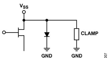
Figure 7. V<sub>SS</sub> Pin Interface Schematic
