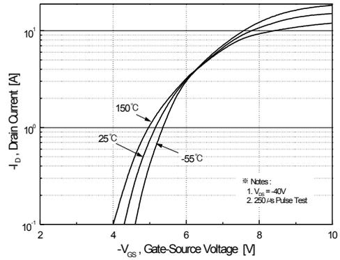
Figure 2. Transfer Characteristics
