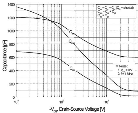
Figure 5. Capacitance Characteristics
