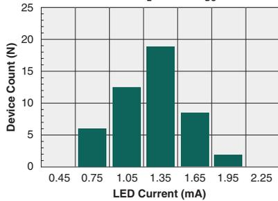
Typical  $I_F$  for Switch Dropout
