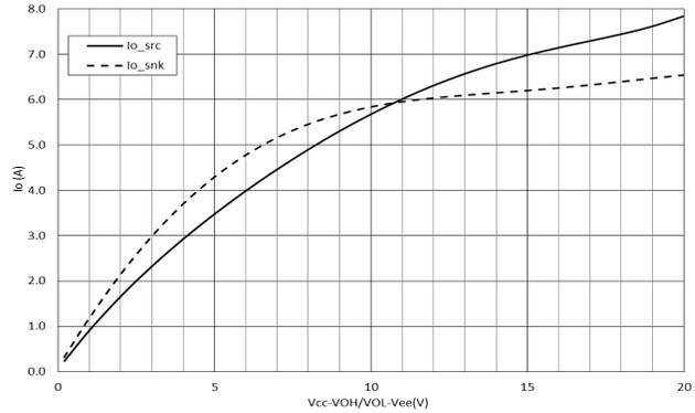
**Figure 19. Output Current vs. Output Voltage Drop**
