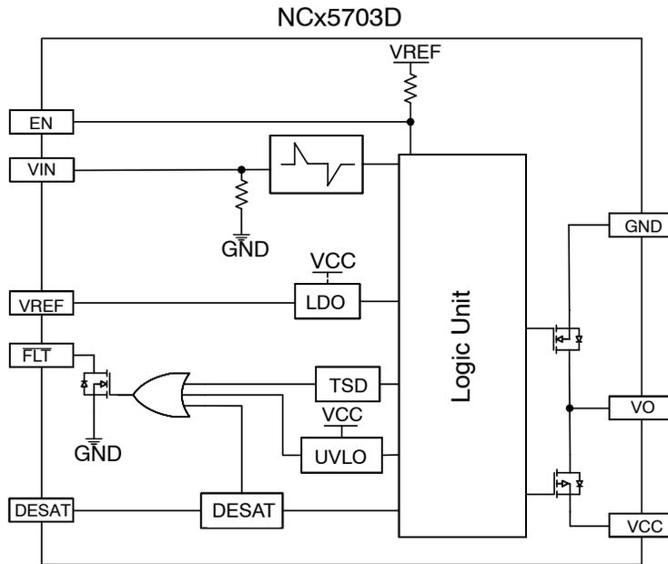
Figure 5(b). Simplified Block Diagram NCx5703D
