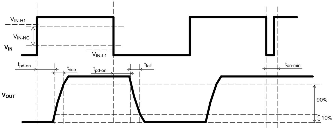
Figure 29. Input and Output Signal Parameters for Opto-coupler
