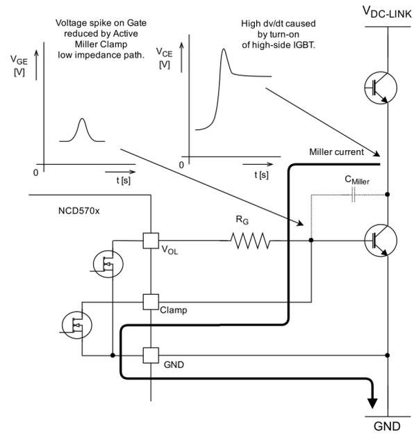
Figure 24. Current Path with Miller Clamp Protection
