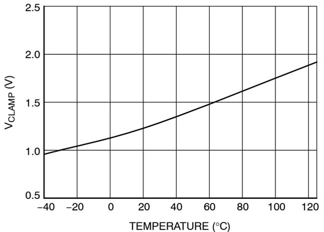
Figure 17.  $V_{CLAMP}$  at 0.5 A (NCx5703A Only)
