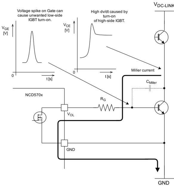
Figure 23. Current Path without Miller Clamp Protection
