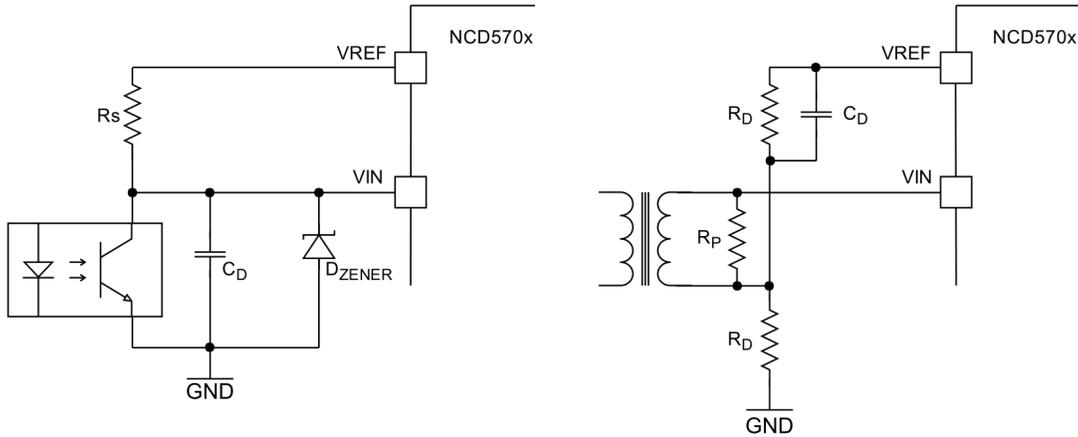
**Figure 27. Opto-coupler or Pulse Transformer At Input**
