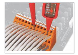
Testing via contact area above the conductors.
