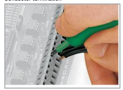
Inserting a conductor via 3.5 mm screwdriver.
