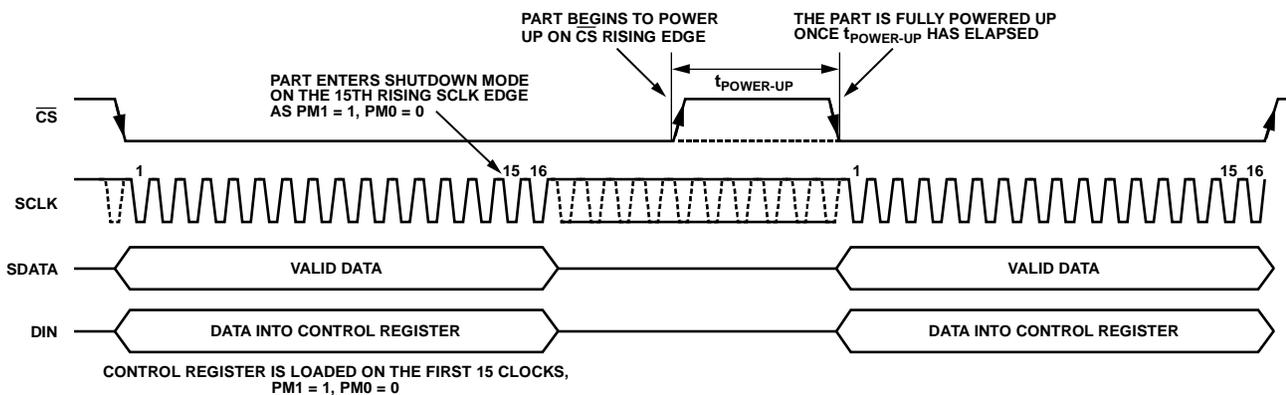
Figure 48. Entering Autoshutdown/Autostandby Mode
