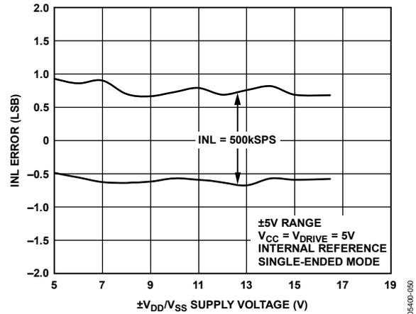
Figure 19. INL Error vs. Supply Voltage at 500 kSPS
