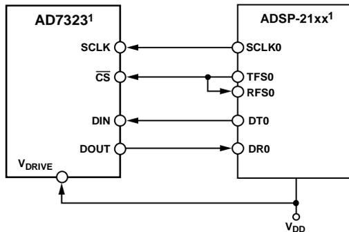
Figure 52. Interfacing the AD7323 to the ADSP-21xx
