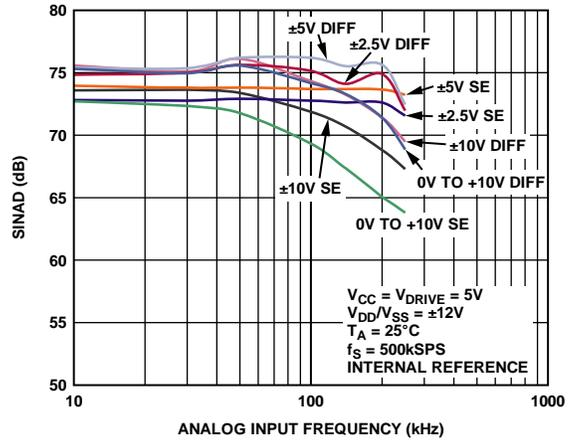
Figure 13. SINAD vs. Analog Input Frequency for Single-Ended (SE) and True Differential Mode (Diff) at 5 V<sub>CC</sub>
