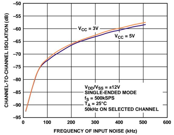
Figure 14. Channel-to-Channel Isolation
