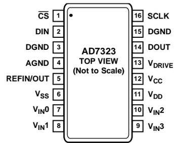
Figure 3. Pin Configuration
