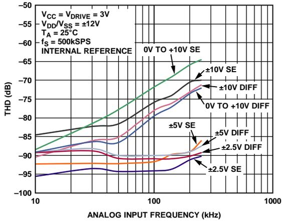
Figure 10. THD vs. Analog Input Frequency for Single-Ended (SE) and True Differential Mode (Diff) at 3 V<sub>CC</sub>
