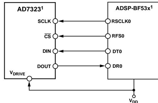
Figure 53. Interfacing the AD7323 to the ADSP-BF53x
