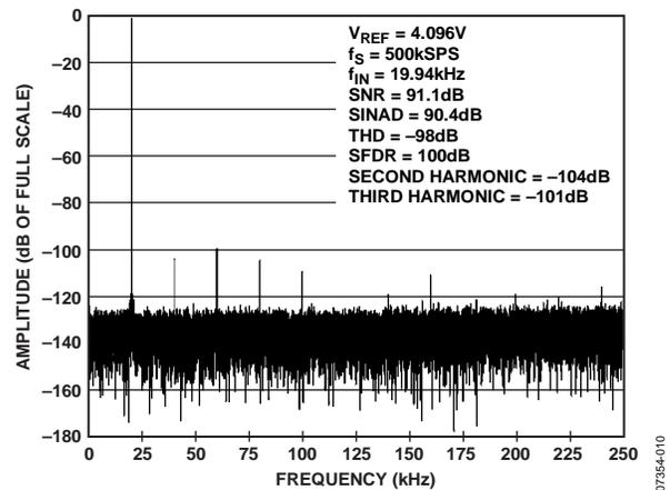
Figure 11. 20 kHz FFT, VREF = 4.096 V
