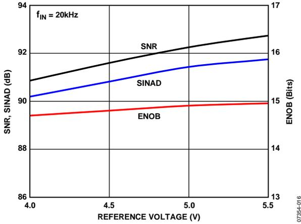
Figure 18. SNR, SINAD, ENOB vs. Reference Voltage
