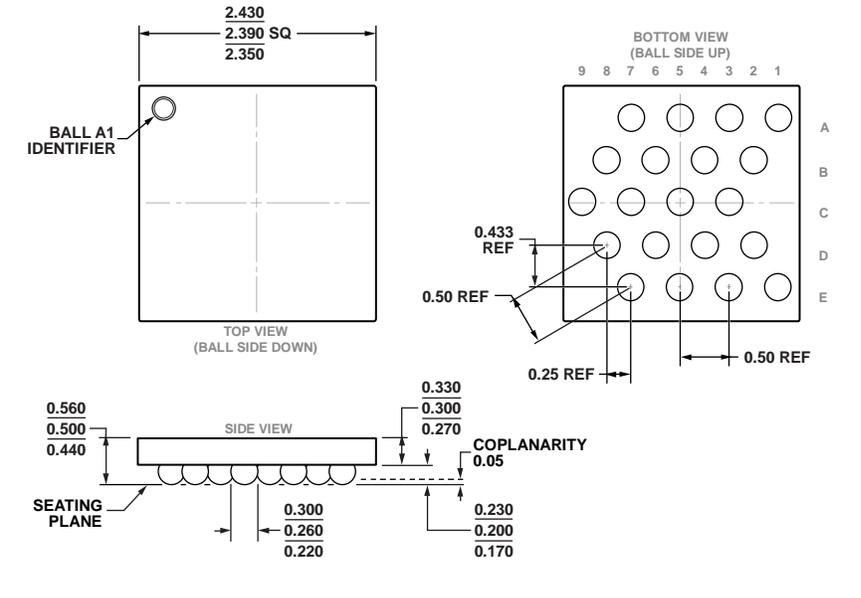
Figure 45. 20-Ball Wafer Level Chip Scale Package [WLCSP]
