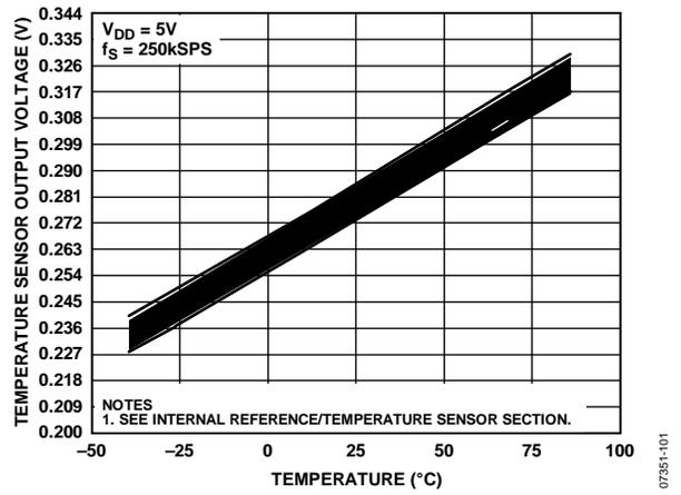
Figure 26. Temperature Sensor Output Voltage vs. Temperature
