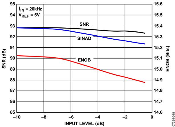
Figure 19. SNR, SINAD, and ENOB vs. Input Level
