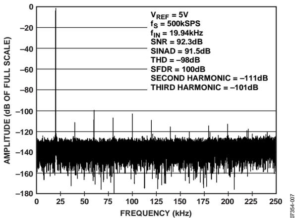
Figure 8. 20 kHz FFT, VREF = 5 V
