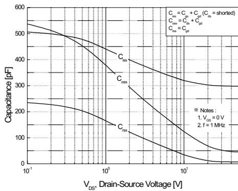
Figure 5. Capacitance Characteristics
