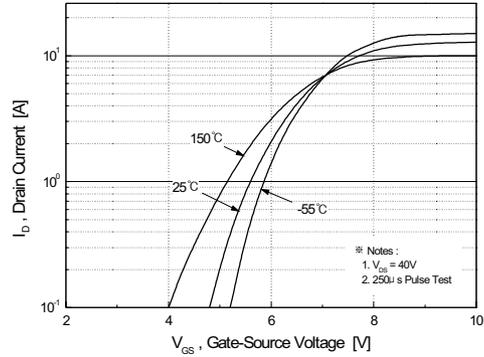
Figure 2. Transfer Characteristics
