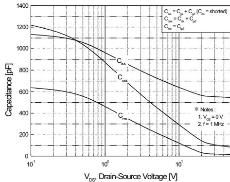
Figure 5. Capacitance Characteristics
