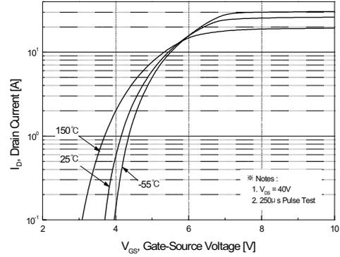
Figure 2. Transfer Characteristics
